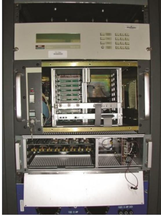
Figure 1.1: First PMU prototype built and designed at Virginia Tech in 1980s
