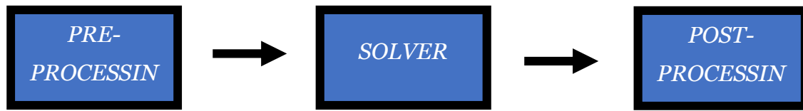
Figure 5.1 :Structure of a CFD software
