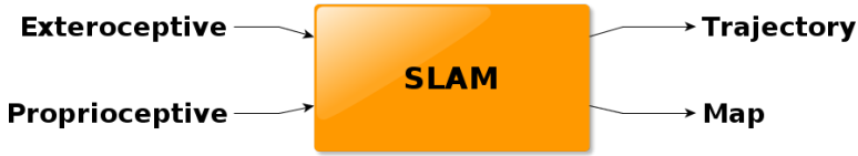
Figure 5.3: The SLAM functional block with its inputs (both proprioceptive and exteroceptive) and outputs (the estimated trajectory and the estimated map).
