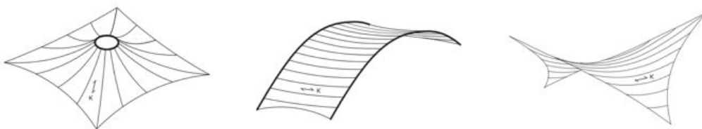
Figure 2.3: Strips layout with warp in the main bearing direction (from Seidel, 2009).
