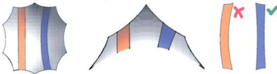
Figure 2.4: Comparison of non-geodesic (orange) and geodesic (blue) cutting pattern generation (from Forster & Mollaert, 2004).
