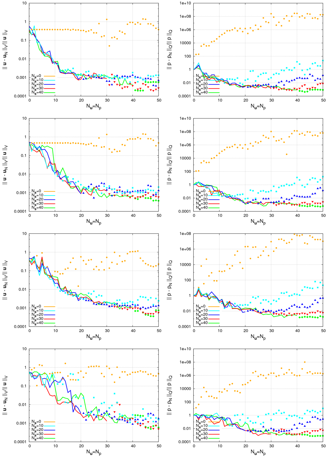
Figure 3.4: Case II – physical and geometrical parameters: error analysis on velocity (left) and pressure (right). From top to bottom: (Re = 90, H_o/H = 1) , (Re = 150, H_o/H = 1) , (Re = 150, H_o/H = 0.5) , (Re = 150, H_o/H = 1.5) .
