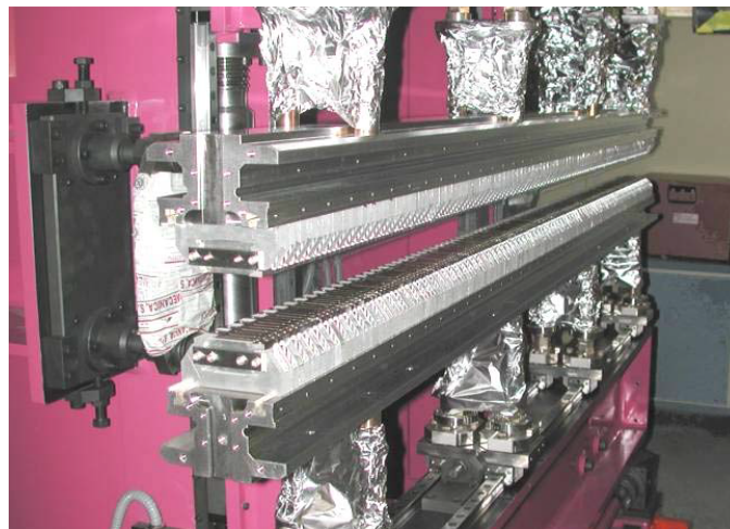
Figure 3.2.2: Photograph of a hybrid U22 undulator. The gap, that is, the distance between upper and lower magnets, is higher than the values which are practically used. [18]
