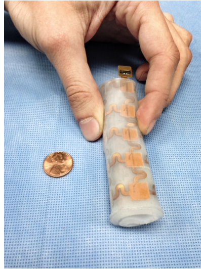
Figure 2.21: The resulted skin extruded from the plastic mold.
