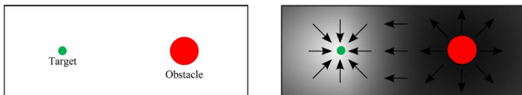
Figure 1.25 Constraints enforced as potential fields. The target acts as an attraction point, while the obstacle acts as a repulsion point (Bowyer, 2014).
