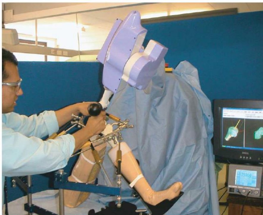
Figure 1.17 "Acrobot" System developed at Imperial College, for Unicodylar Knee Arthroplasty (UKA).
