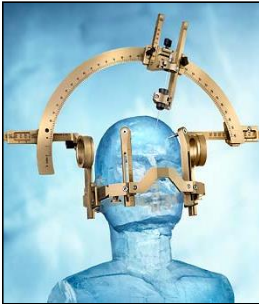
Figure 1.5 Stereotactic frame for the mapping procedures of the target points within the skull.
