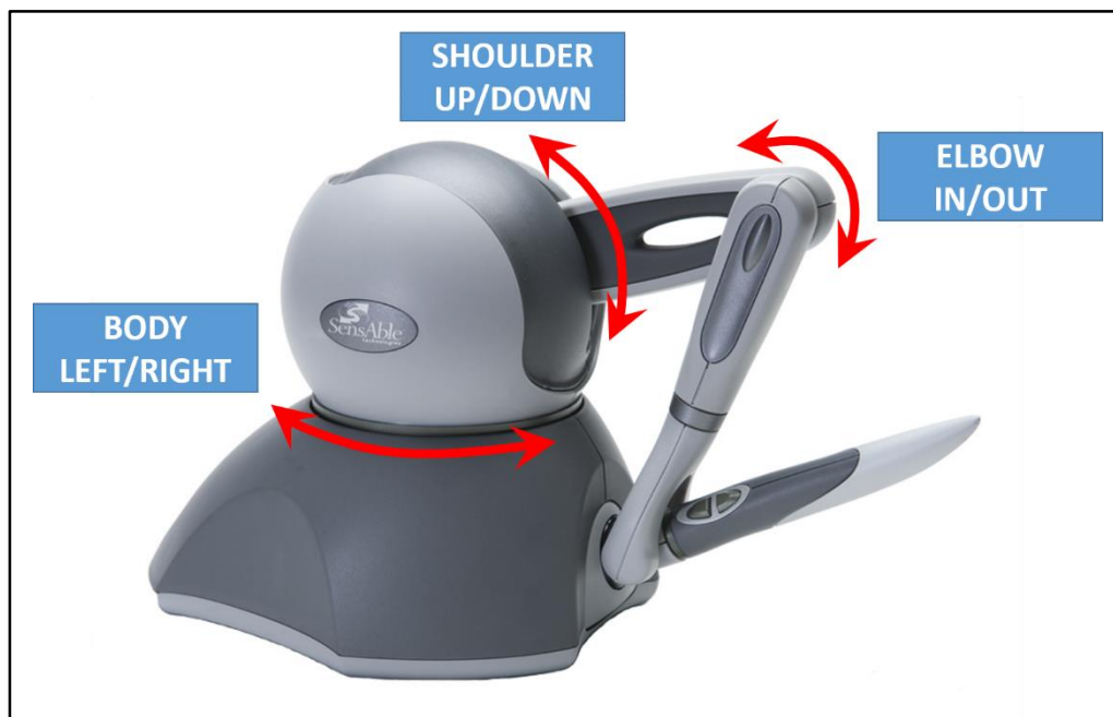
Figure 2.18 Phantom OMNI® haptic device. It is characterized by six degrees of freedom positional sensing and three torque actuators that control the angular position of the body, the shoulder and the elbow of the device.
