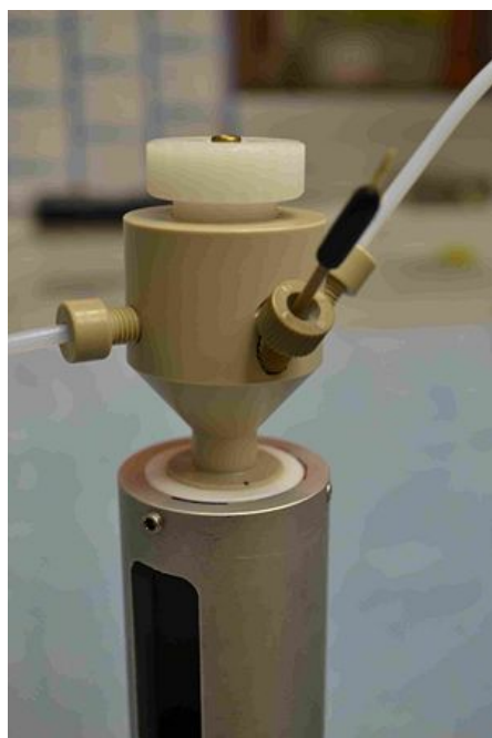
(a) Flow cell mounted on the diffractometer.
