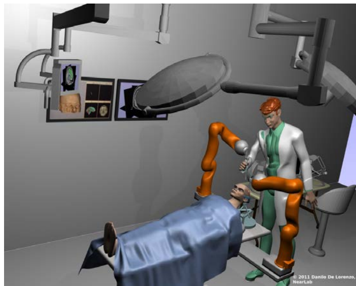
Figure 1.4 Hands-on scenario for open-skull neurosurgery. The surgeon manually guides the surgical instruments, fixed to the robotic assistant, and operates next to the patient.
