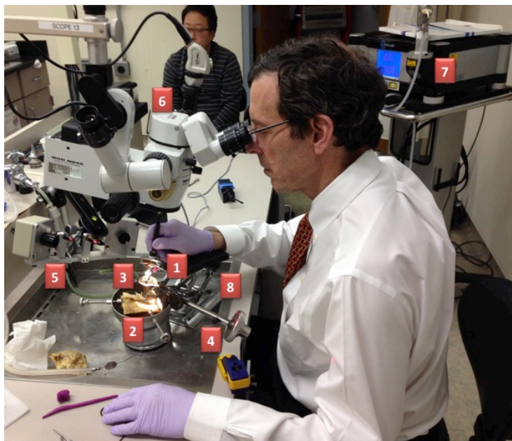
Fig. 6.3: Experiments setup. All the components can be seen: 1) Micron, 2) target (bone in this case) and bone holder, 3) speculum, 4) speculum holder, 5) ASAP, 6) microscope, 7) laser machine, 8) hand rest.
