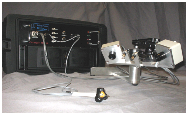
Fig. 4.2: Micron system components: hand piece, electronics and PSD cameras (part of the ASAP apparatus).
