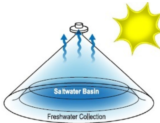
Figure 2.6: Schematic layout of a basic solar still [44]
