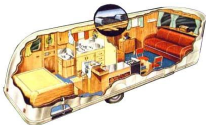
Fig.3.2.6. (Left) Spartan Manor, 1946, 3d section. Source [ http://www.spartantrailer.com/restoration.html (accessed 4th July 2013)]; Fig.3.2.7. (Right) Kitchen cabinet/dining table in closed (40 cm x 71cm /h73) and open position (132 cm x 71 cm /h73 cm) Spartan Manor, from 1946. Source [ http://www.spartantrailer.com/restoration.html (accessed 4th July 2013)]
