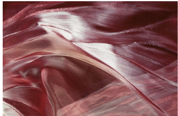
Fig.5.1.4.6. Phenomena fabric made of combination of stainless steel + copper, by AlphaMesh, Germany. Picture source: [http://www.alphamesh.de/index.php?page=vision-2 (accessed 12 th November 2013)]
