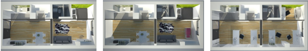
Fig.5.1.1.3. Functional changeability of layout where kitchen and bathroom units are immobile. Case study 52: Garage project by Damir Spoljar, Zagreb, 2009.
