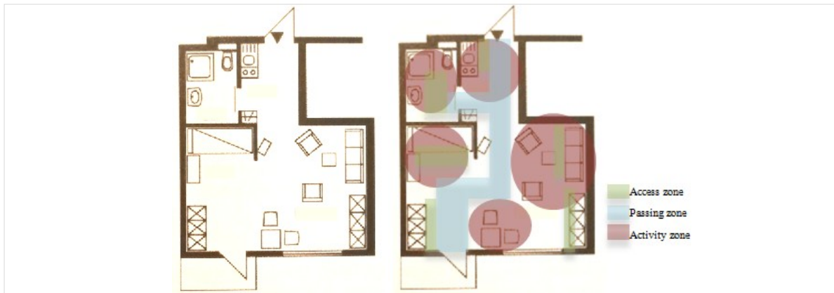
Fig.8.4.1.2. (Left) One room flat (40 m 2 ). Source: “Bauenwurfslehre: Grundlagen, Normen, Vorschriften” (Neufert et al. 2005). Fig.8.4.1.3. (Right) Relation between access zone, passing zone and activity zone in one room flat (40m 2 ).
