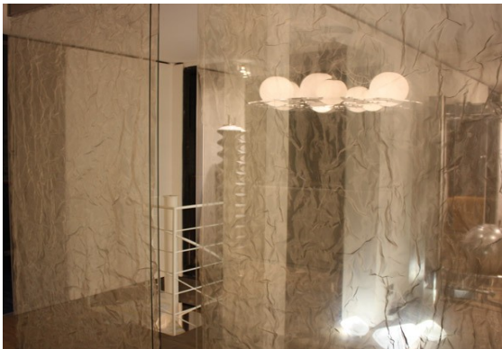
Fig.5.1.4.5. Fabric created by weaving technology with finely spun stainless steel yarns lending the fabric a restrained elegance for unique moulding and shaping properties, by AlphaMesh, Germany. Picture source: [http://www.alphamesh.de/index.php?page=seda-2 (accessed 12 th November 2013)]
