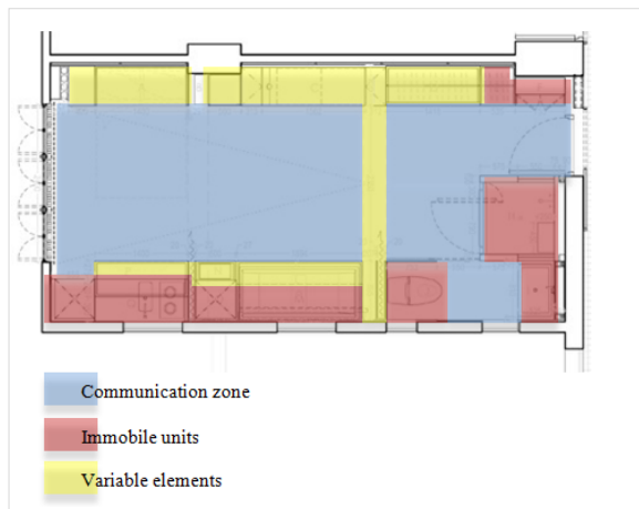
Fig.8.4.2.5. Relation between communication zone, immobile units and variable elements.
