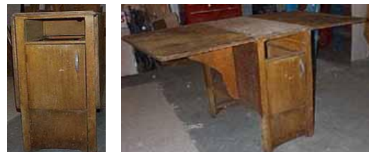
Fig.3.2.6. (Left) Spartan Manor, 1946, 3d section. Source [ http://www.spartantrailer.com/restoration.html (accessed 4th July 2013)]; Fig.3.2.7. (Right) Kitchen cabinet/dining table in closed (40 cm x 71cm /h73) and open position (132 cm x 71 cm /h73 cm) Spartan Manor, from 1946. Source [ http://www.spartantrailer.com/restoration.html (accessed 4th July 2013)]
