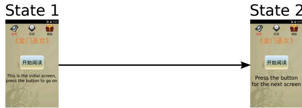
FIGURE 3.4: State 2 is a stuck node. When reached the edge from state 1 to state 2 is removed and the application restarted. The application will restart from state 1 which now is a stuck node.
