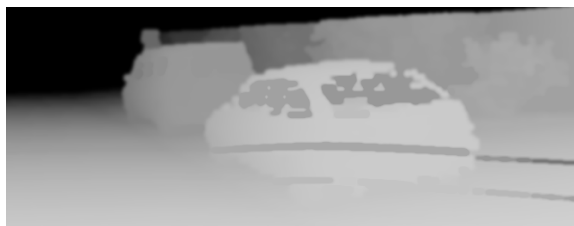
Figure 3.4: Depth image rendered from HDL-64E data. Note the visible gap between the two laser banks.
