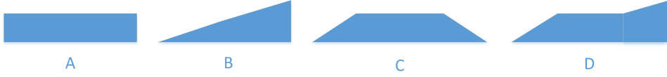
Figure 4.5: Various types of slopes. The slope type A and type B is indistinguishable by the Velodyne. The ground on slopes of type C and D cannot be extracted by a plane segmentation
