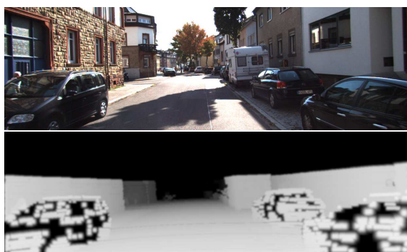
Figure 3.5: Problem in acquiring range distances on dark materials. Note the corresponding missing depths on black cars.
