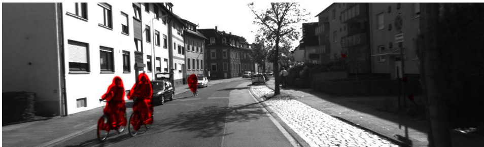
Figure 6.13: A change mask applied to the red channel in a grayscale image.
