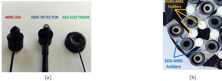
Figure 3.3: (a) Sensors, from left to right: NIRS LED, NIRS Si photodiode, EEG Ag/AgCl passive electrode. (b) EEG-NIRS laser-cut holders (pointed by blue arrows) and NIRScout holders (ocra arrow) between NIRS sensor plastic spacers.
