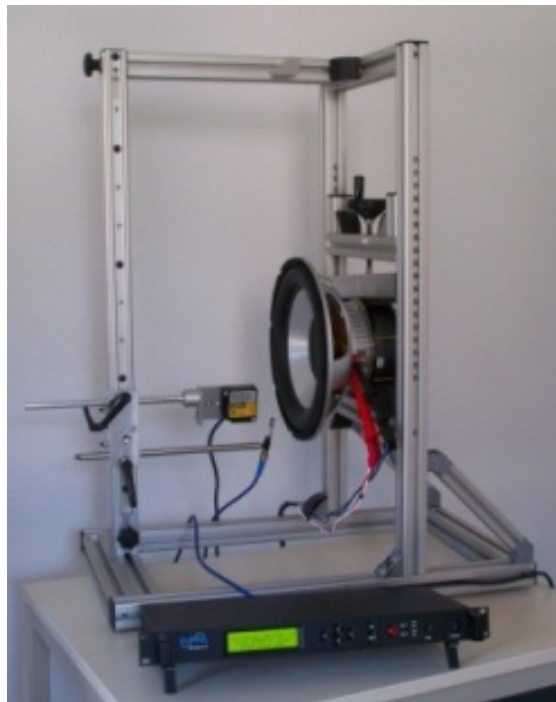
Figure 5.1: Full setup of the Distortion Analyzer in the free air mount configuration.
