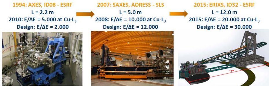
Fig. 3.3: Pictorial view of the historical evolution of soft x-rays RIXS spectrometers. Corresponding dimensions and resolving power at Cu-L 3 are indicated.
