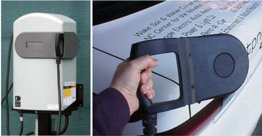
Figure 3.22: Small paddle inductive station (Left), and the paddle (Right)
