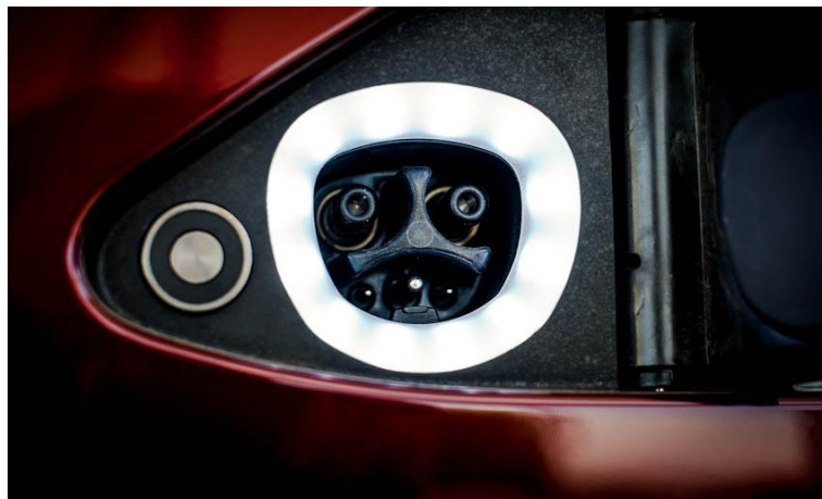
Figure 3.3: Tesla Model S charging port on USA car
