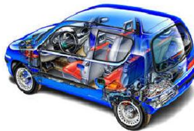
Figure 2.5: Cutaway view of the FIAT Seicento Elettra
