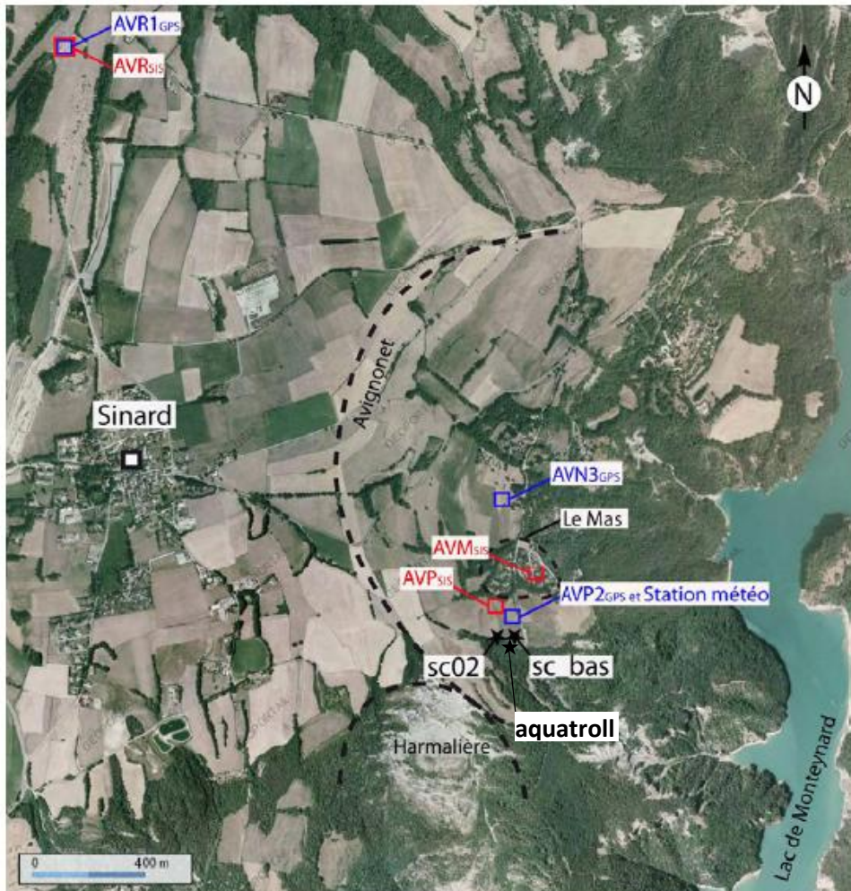
Figure 5 – Monitoring instruments location.
