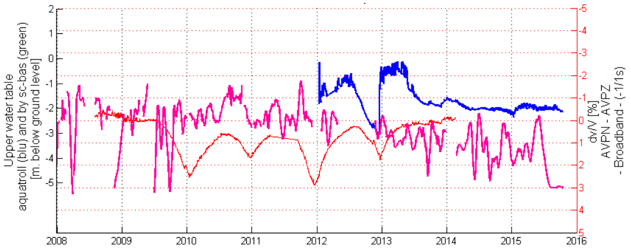
Figure 58 - Comparison between dv/V ( AVP_N - AVP_Z , Broadband) and piezometry. Comparison between Broadband (purple) and upper-perched water table level measured by aquatroll (blu) and by sc_bas (green) in AVP_N - AVP_Z .
