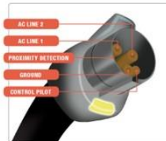
Figure 23: SAE J1772 Type connector
