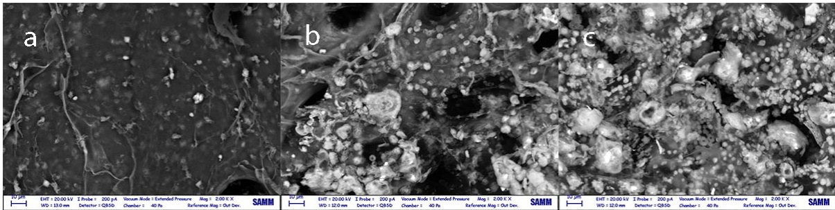
Figure 3-36: SEM images of CH+30% Bioglass small size at magnification 2000x after a) 7days, b) 14days, and c) 28days
