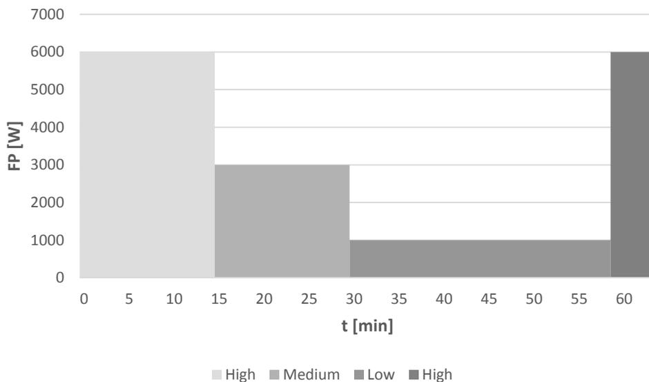
Figure 3.7.4 – Example of a burn cycle resulting from the combination of two cooking tests, adapted from Pemberton-Pigott [83]; high, medium and low represent firepower levels.
