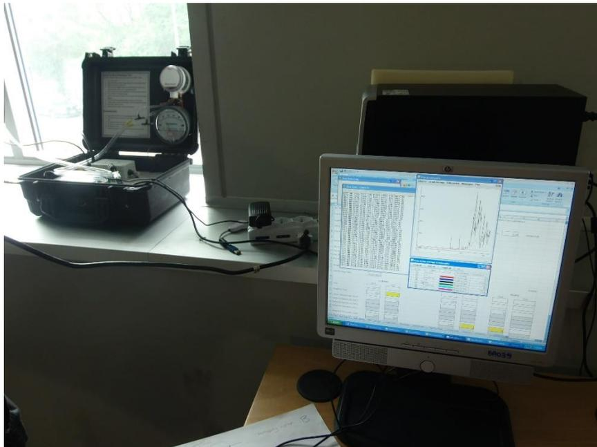
**Figure A 2** – PEMS Sensor Box and real-time data output to the computer.
