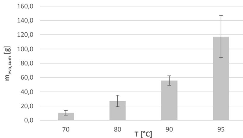
**Figure 4.3.13** – Cumulative mass of water vaporised at different temperatures, lid-off case. Bars represent extended uncertainty.
