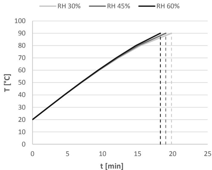
Figure 4.3.1 – Temperature trends over time for different values of ambient RH.
