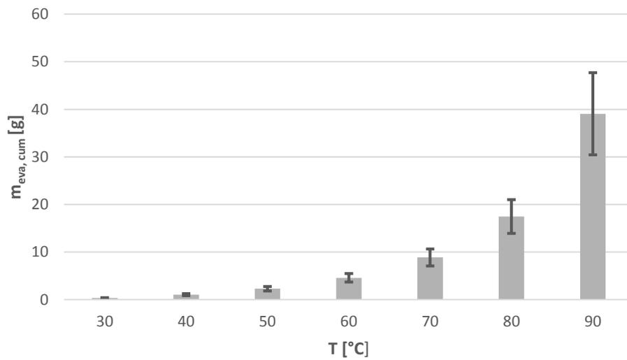
**Figure 4.3.6** – Average values of cumulative mass of water vaporised at different temperatures for a simulation of 7 test replicates, each varying 5% RH from the previous. Bars represent standard deviations.
