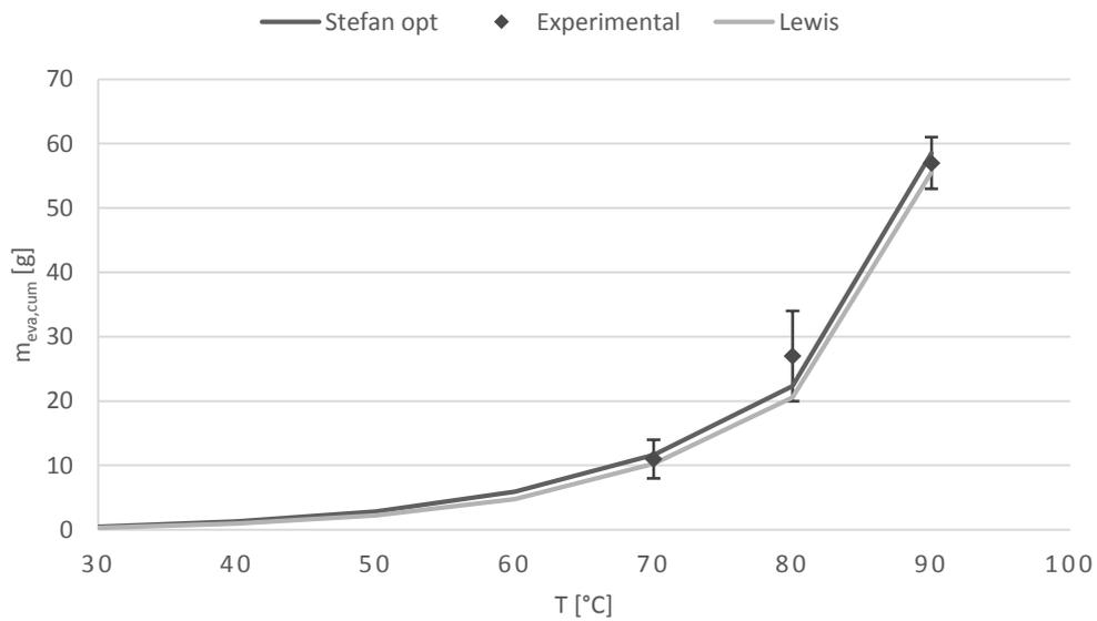
**Figure 4.2.7** - Cumulative mass of water vaporised at different temperatures for Lewis and modified Stefan models and for experimental data; bars represent standard deviation.
