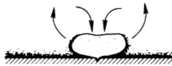
**Figure 4.4.2** – Bubble growth in subcooled liquid: steam condenses on the top, while evaporation continues on the bottom, determining bubble collapse. Dark regions represent locally superheated liquid. Adapted from Lienhard et al. [94].
