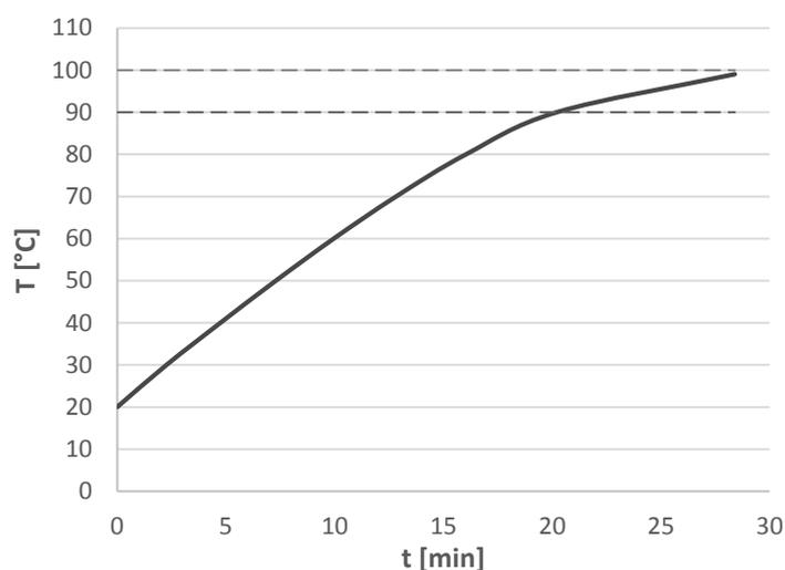
**Figure 4.4.6** – Temperature trend over time for water in a cooking pot heated by a constant heat source, with no lid or any other form of insulation.
