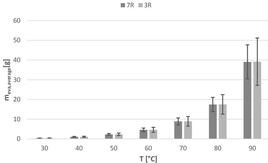
**Figure 4.3.8** – Comparison of total mass of water vaporised at different temperatures between a 7 replicates simulation and a 3 replicates simulation. Bars represent standard deviations.
