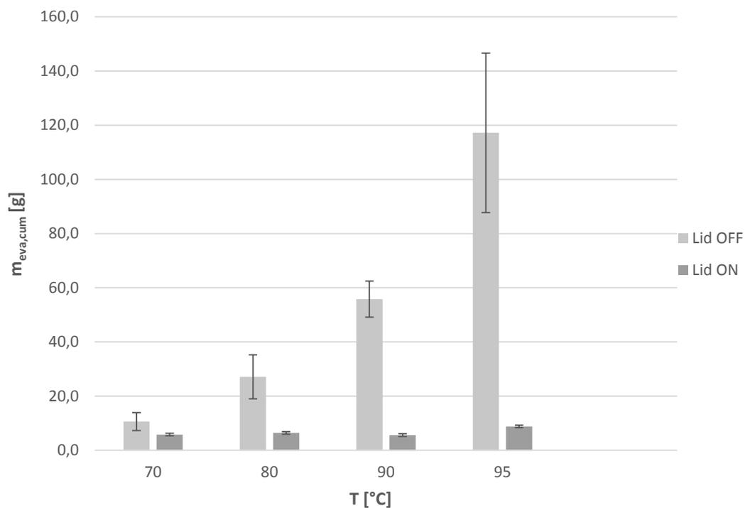
**Figure 4.3.14** – Comparison of cumulative mass of water vaporised at different temperatures between the lid-on and lid-off cases. Bars represent extended uncertainty.
