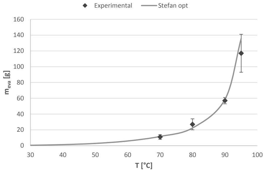
**Figure 4.4.3** – Cumulative mass of water vaporised at different temperatures, comparison between the optimised Stefan model and experimental data (electric heater). Bars represent standard deviations.
