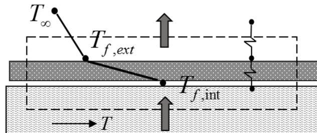
**Figure 4.4.5** – Heat flux and temperatures between the water surface and the insulating layer.
