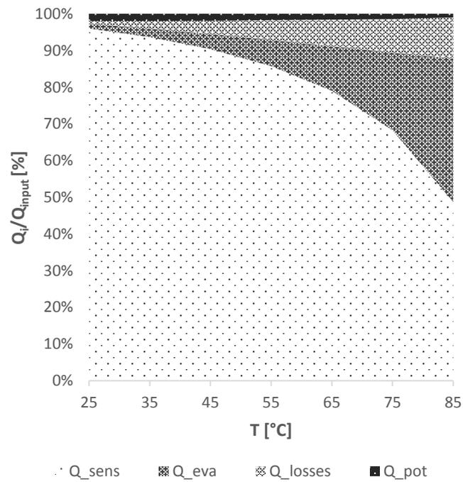
**Figure 4.3.2** – Distribution of thermal power fractions as a function of temperature, for RH 30%.
