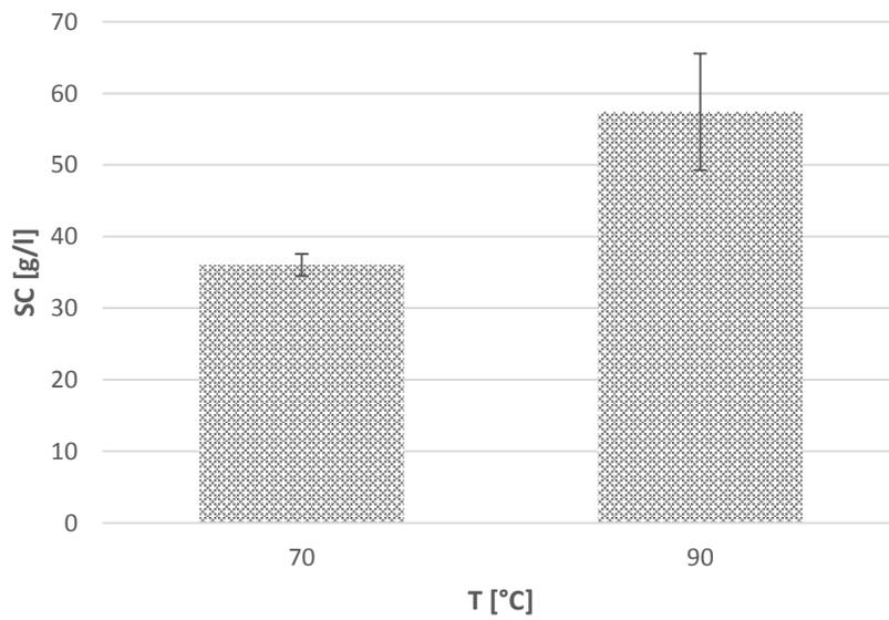
**Figure 4.3.10** – Average values of specific fuel consumption for a simulation of 3 replicates, at 70 and 90°C. Bars represent combined uncertainty for a 95% CI
