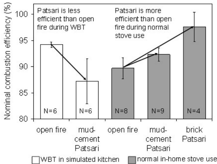
**Figure 2.2.1** – Comparison of nominal combustion efficiencies of different stove types, referred to WBT and field measurements. Source: Johnson et al. [74].
