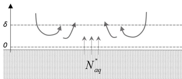
**Figure 4.2.1** – Sketch of the mass concentration boundary layer as a stagnant film. The subscript “aq” indicates water.
