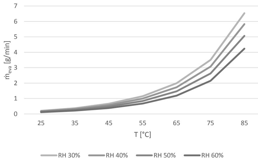
**Figure 4.2.8** – Rate of evaporation as a function of water temperature for different values of indoor relative humidity.
