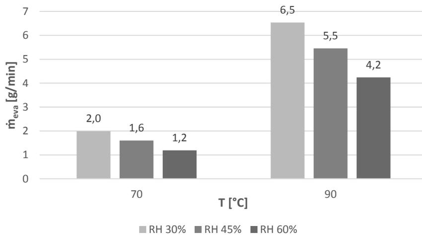
Figure 4.3.4 – Variations in the rate of vaporisation at 70 and 90°C for different values of RH.
