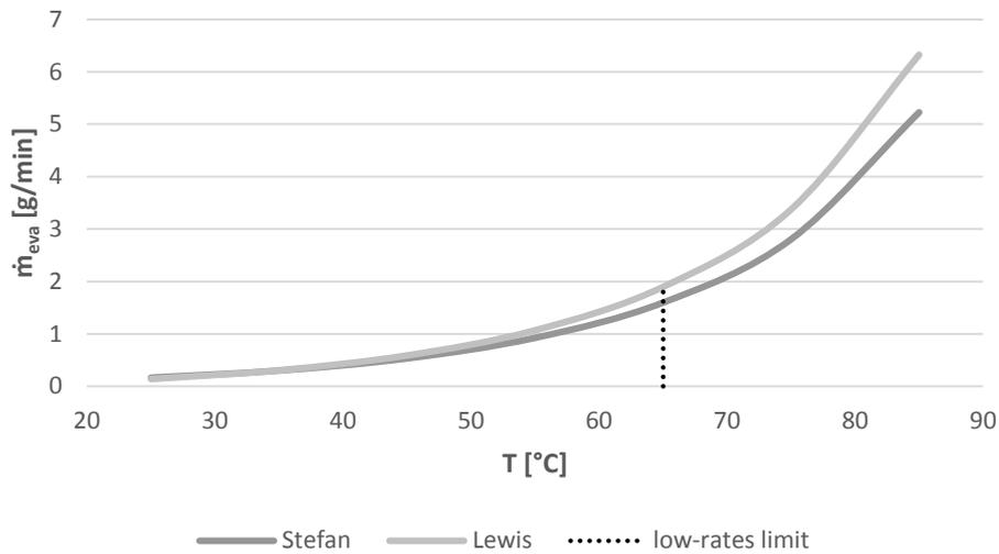
**Figure 4.2.3** – Evaporation rates comparison for Stefan and Lewis models, at different temperatures.
