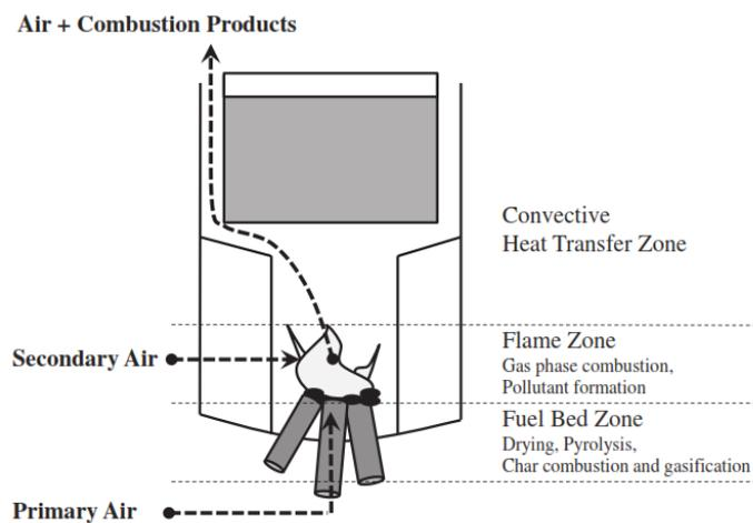
**Figure 1.2.3** – Typical wood ICS design, with different processes highlighted; source MacCarty et al. [34].
