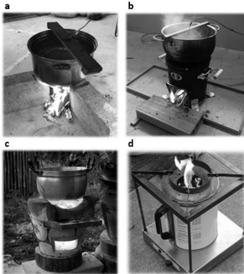
**Figure 1.2.4** – Examples of different cookstove designs. a) three-stone fire; b) rocket-type wood ICS; c) charcoal stove; d) forced-draft gasifier.<sup>1</sup>
