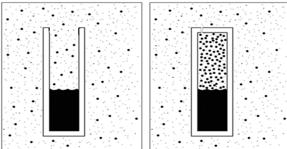
**Figure 4.3.11** – Container filled with water in a humid air environment before and after placing a lid on its top; source: Sidebotham [95].
