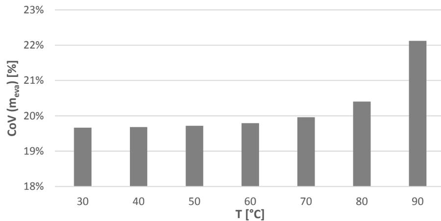
**Figure 4.3.7** – Coefficient of variation for the cumulative mass of water vaporised at different temperatures for a simulation of 7 replicates, each varying 5% RH from the previous.
