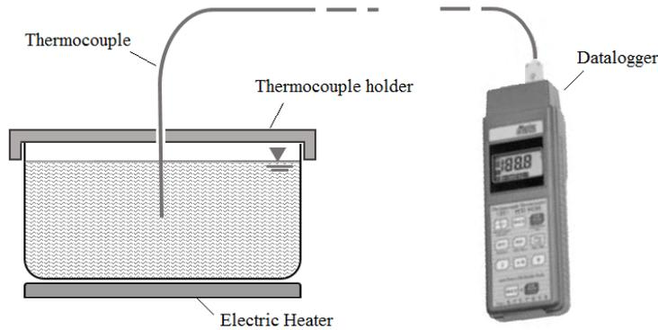
**Figure 4.3.12** – Simple sketch of the experimental set-up.
