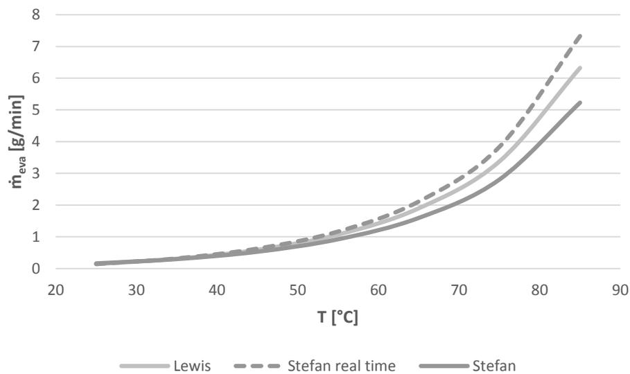
Figure 4.2.5 – Evaporation rates comparison for Lewis, Stefan and real-time Stefan models, at different temperatures
