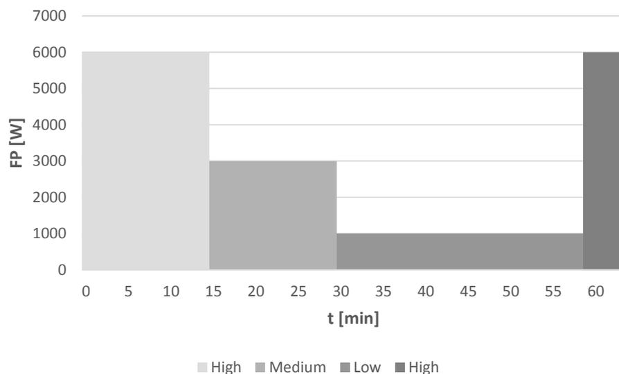
**Figure 4.4.7** – Example of a burn cycle resulting from the combination of two cooking tests, adapted from Pemberton-Pigott [83]; high, medium and low represent firepower levels.
