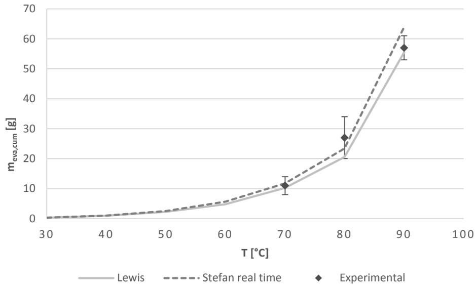
**Figure 4.2.6** – Cumulative mass of water vaporised at different temperatures for Lewis and real-time Stefan models and for experimental data; bars represent standard deviation.
