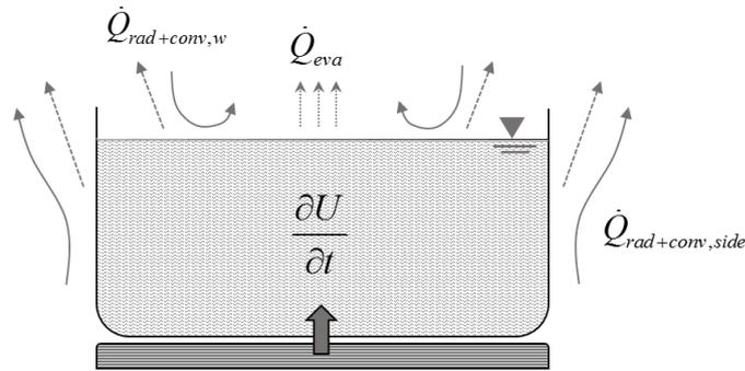
**Figure 4.2.9** – Sketch of the heat transfer model for a cooking pot filled with water and subject to a constant heat source.
