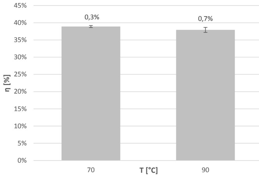
**Figure 4.3.9** – Average values of thermal efficiencies for a simulation of 3 replicates, at 70 and 90°C. Bars represent combined uncertainty for a 95% CI
