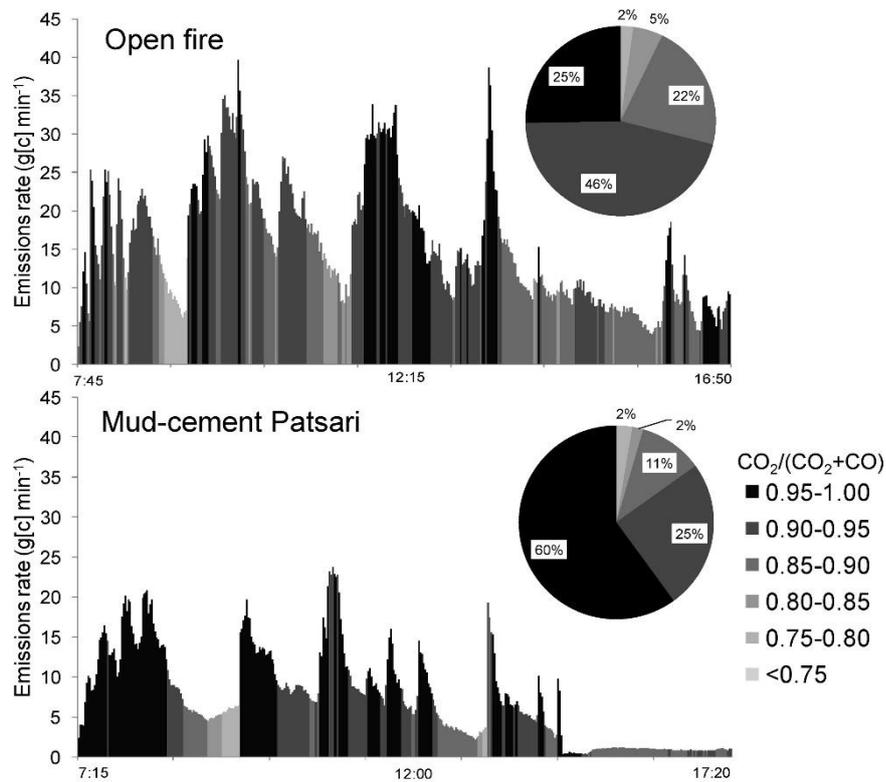
**Figure 3.7.1** – Minute by minute emission rates and  $\text{CO}_2/(\text{CO}_2+\text{CO})$  ratio for open fire and Mud-cement Patsari, adapted from Johnson et al. [68].
