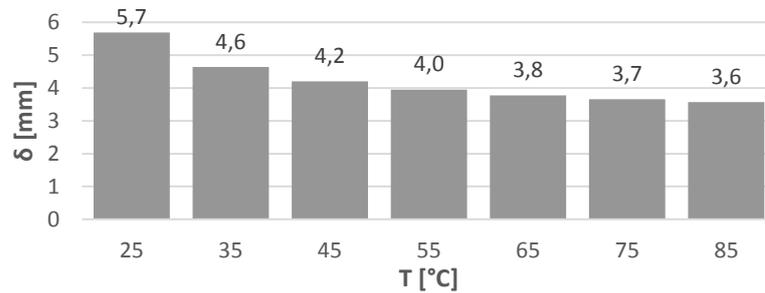
Figure 4.2.4 – Mass transfer boundary layer thickness at various temperatures.
