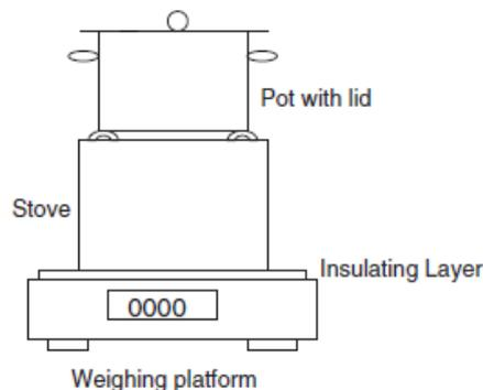
**Figure 3.6.1** - HTP experimental set-up, adapted from Makonese et al. [84].
