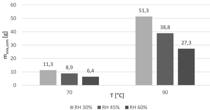
**Figure 4.3.5** – Variations in the total mass of water vaporised at 70 and 90°C for different values of RH.
