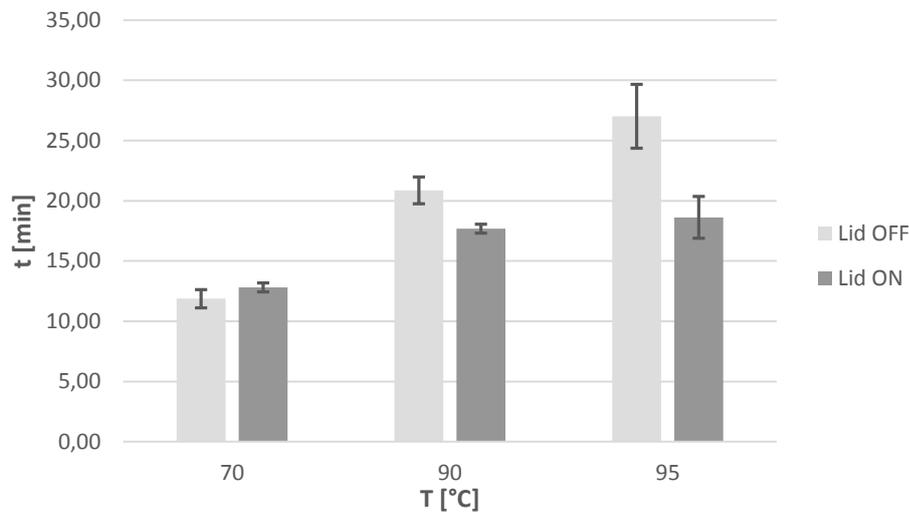
**Figure 4.3.15** – Comparison of averaged values for the test ending time at different temperatures for the lid-off and lid-on cases. Bars represent standard deviation.
