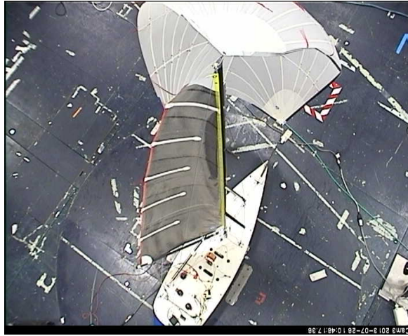
Figure 6.9: Gennaker flying shape and forces variation with trim.
