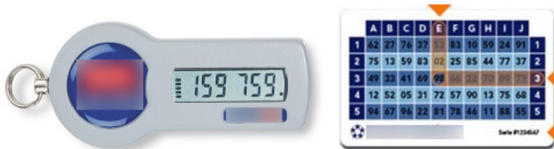
Figure 3: Example of weak authorization mechanism with OTP-token (or TAN) [6]
