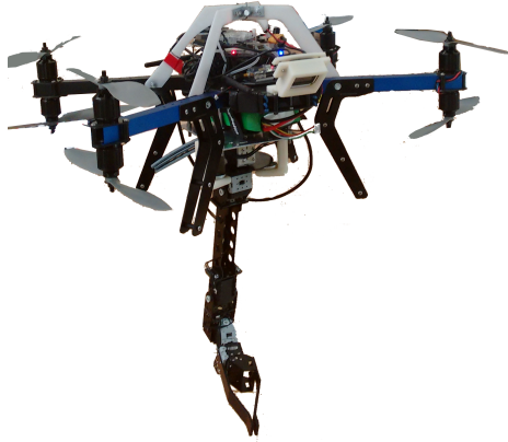
Figure 3.12: Aerial manipulator, used in the experiments, consisting on a 3DR-X8 coaxial multirotor platform with a custom-built 4 degrees-of-freedom serial arm attached below.
