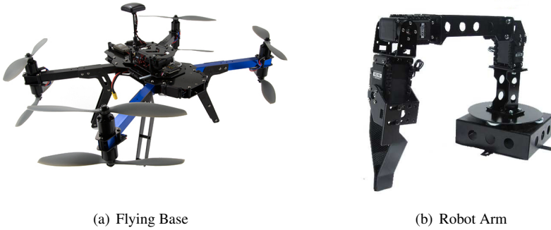
Figure A.2: The image on the left represents the chosen flying base, a 3DR X8+ coaxial octacopter. On the right is it shown the CrustCrawler robotic arm, which has been assembled to be mounted underneath the flying base.
