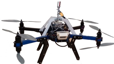
(c) Support for the quadrotor, used to sustain the system preventing crashes.
