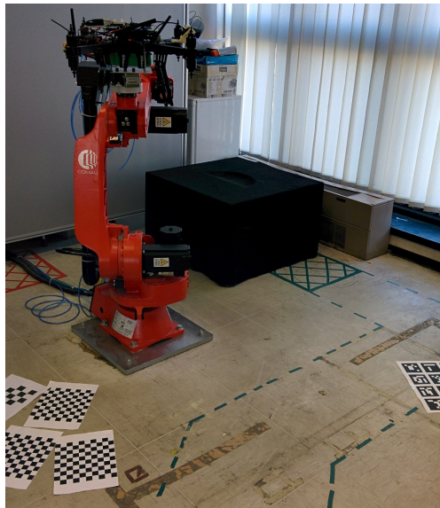
Figure 4.4: Experimental Set-Up. A quadrotor is fixed to the end effector of the Comau Smart Six and a marker is on the ground.
