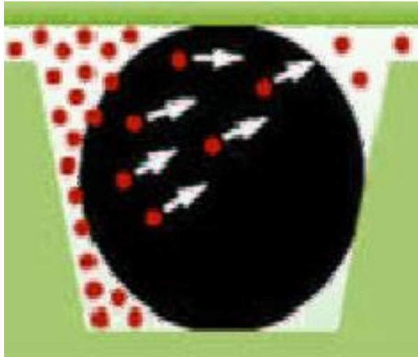
Figure 12: Permeation of a polymeric spherical element inside a vacuum system
