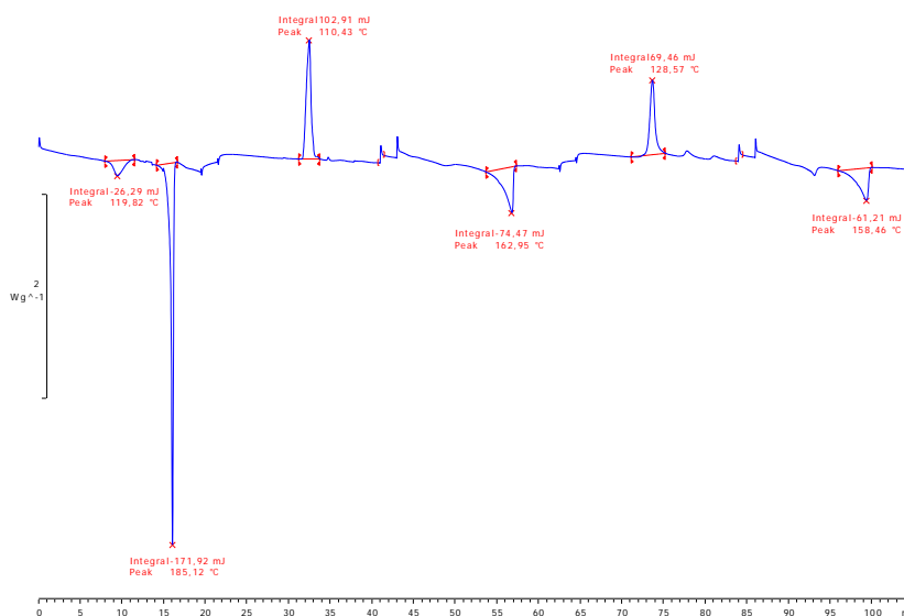
Figure 7.2.3 DSC curves of complex 1-12-2-6 measured at a heating rate of 10 ^{\circ}\text{C}/\text{min} under flowing nitrogen atmosphere.
