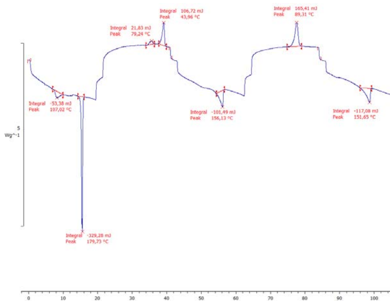
Figure 7.2.2 DSC curves of complex 1-10-2-4 measured at a heating rate of 10 ^{\circ}\text{C}/\text{min} under flowing nitrogen atmosphere.
