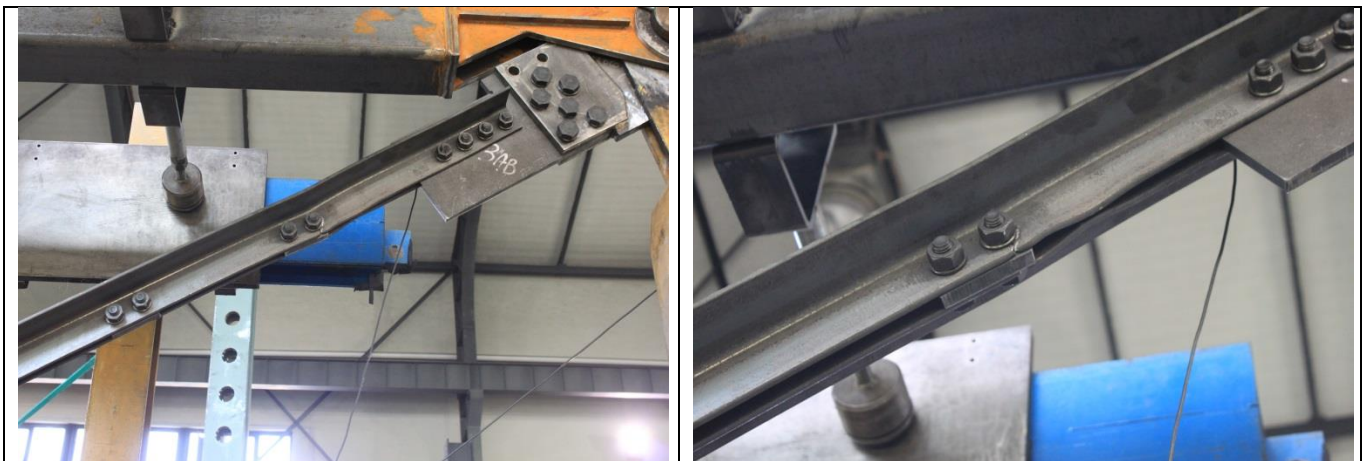
Figure 152. Detail of plastic hinge on continuous brace.
