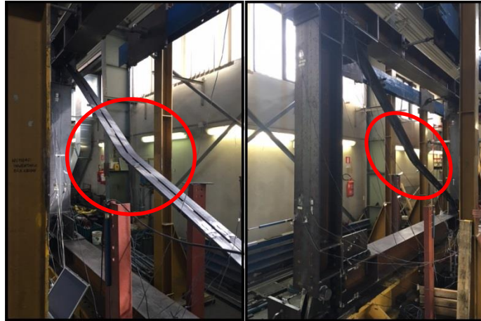
Figure 92. Test 7: plastic hinge during post-buckling phase (0.62% of drift)
