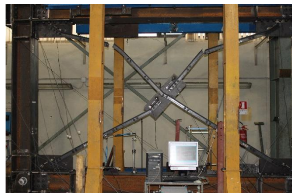
b. After both bracings completely fractured
