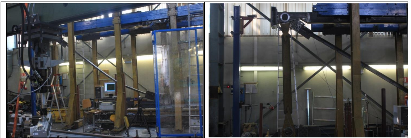
Figure 164. Buckling of diagonal. (+0.19% drift applied)
