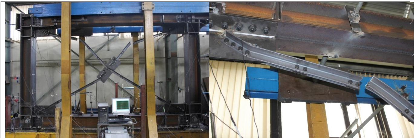
Figure 124. Failure at mid-span of the north-west continuous diagonal (first frame compression peak of \pm 38 mm cycle).
