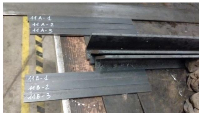
Figure 17. Samples extracted from angular profiles of the braces for tensile tests
