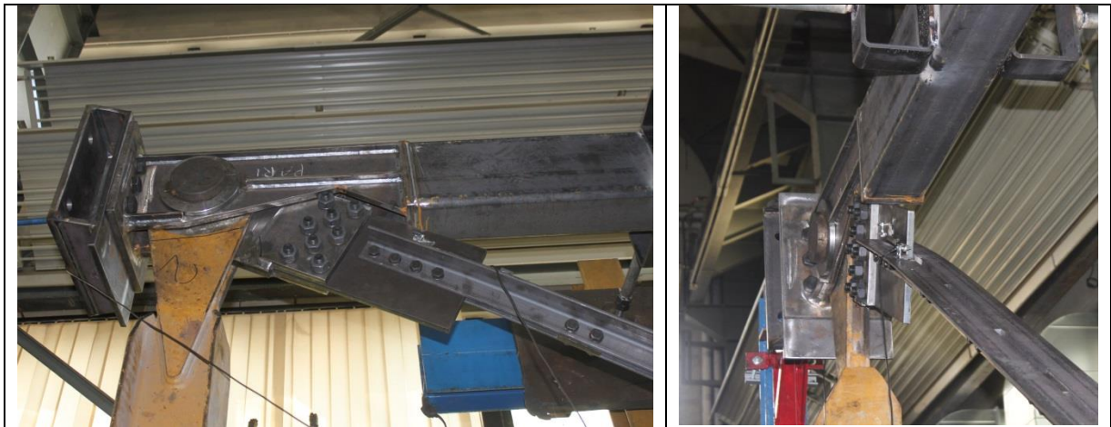
Figure 144. Buckling mechanism of the system. Brace touched the beam..
