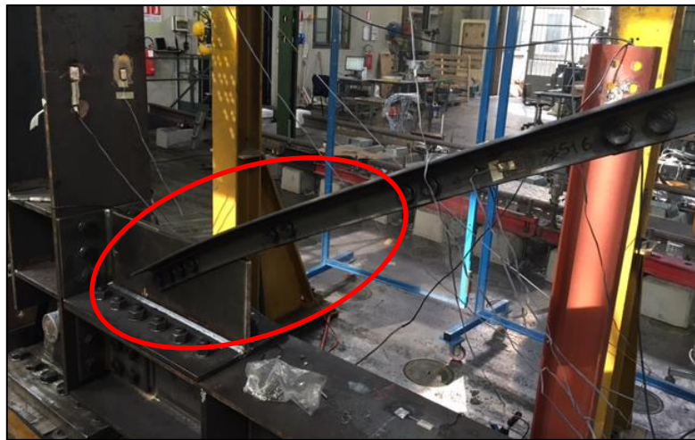
Figure 93. Test 7: plasticization of diagonal edge (0.62% of drift)
