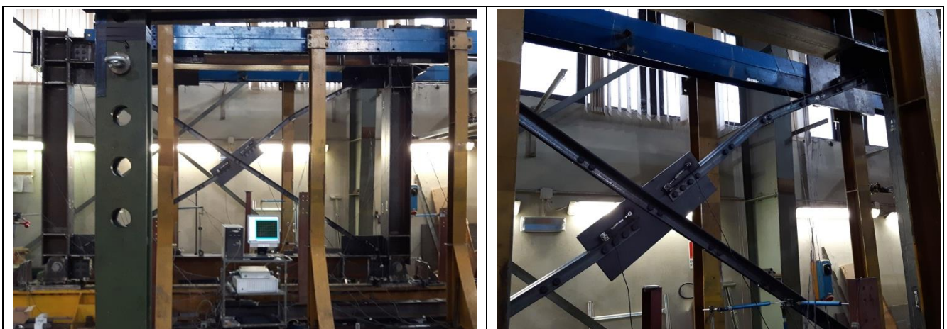
Figure 115. 5. Plastic hinge formed after first in-plane buckling on mid-span of NE diagonal
