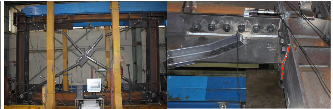
Figure 126. Frame at test end; yielding at gusset.
