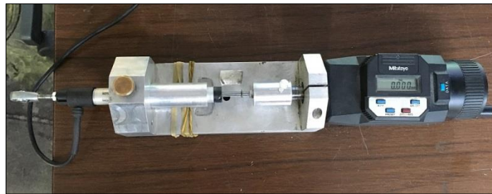
Figure 47. Calibration of a potentiometer through digital micrometer
