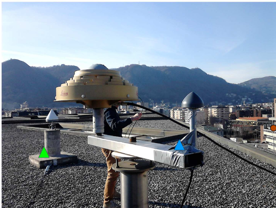
Figure 4.14 – The reference stations in Experiment 3: Como EUREF (green triangle) and secondary reference station (blu triangle); the orange circle is in correspondence of rover position
