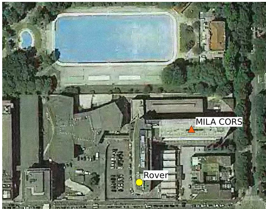
Figure 2.6 – The positions of MILA CORS (Red triangle) and the rover (yellow circle); the distance of the two points is less than 80 meters.
