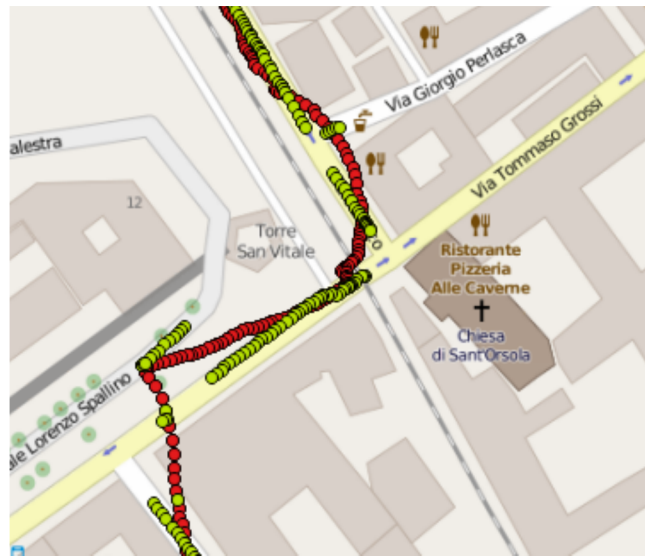
Figure 3.6 – Correction on the nearest segment: the reds circles are positions of the points collected, the green circles are the positions after the correction to the nearest path
