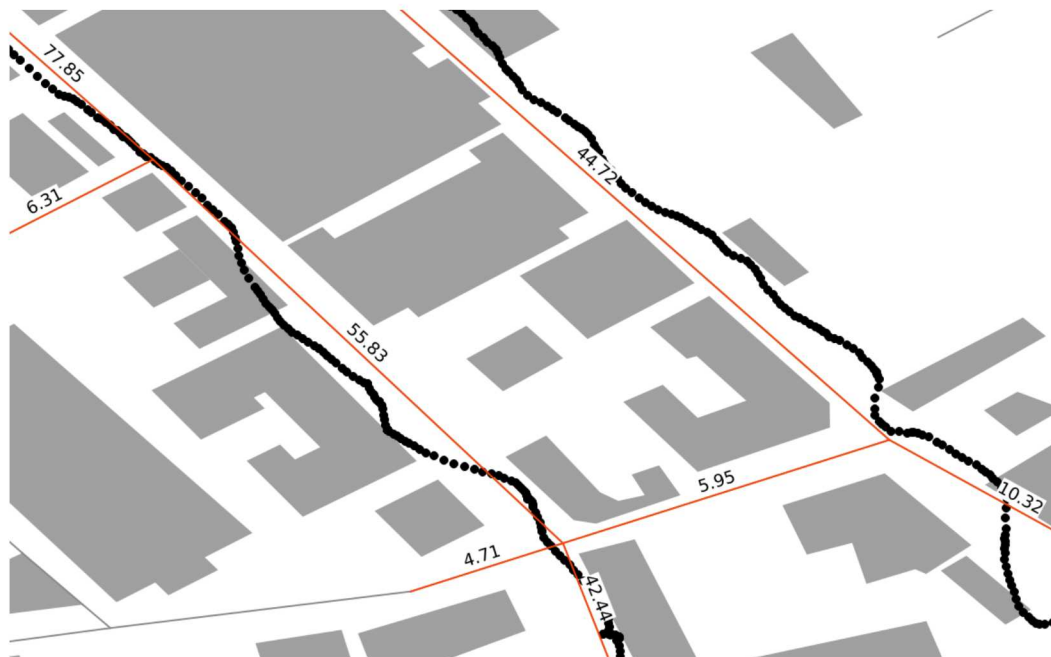
Figure 3.18 – The red lines are the candidate segments with the score received, black circles are the estimated points - Day 14-259
