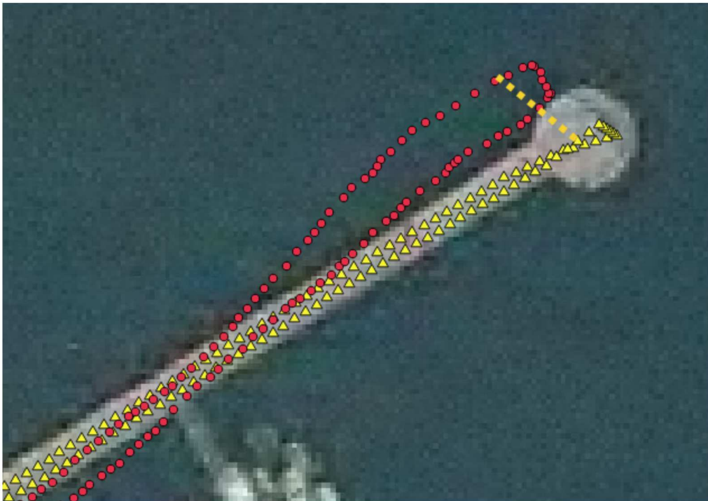
Figure 2.21 – Yellow triangles are the points estimated with the geodetic receiver, red circles are the positions collected with the low cost receiver during the same survey. The different of positioning between points at the same epoch is the error (the orange dotted line)
