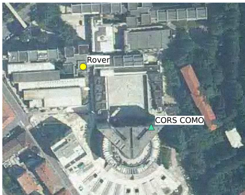
Figure 2.7 – The positions of COMO CORS (Green triangle) and the rover (yellow circle); the distance of the two points is less than 150 meters.
