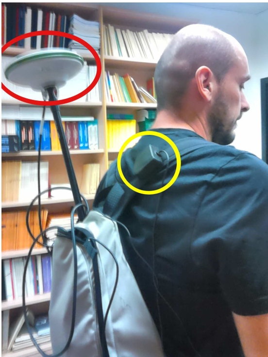
Figure 2.20 – The position of geodetic antenna (red circle) and u-blox antenna (red circle) during the test; smartphones was taken by hand
