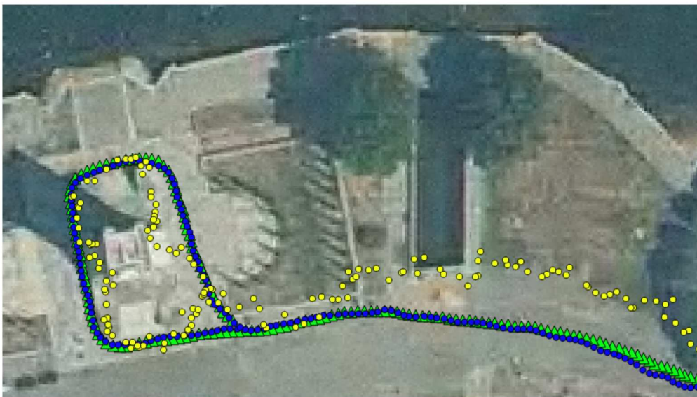
Figure 2.29 – Detail of the area near War Memorial: points collected with geodetic receiver (green triangles), u-blox (blue circles) and smartphone (yellow circles) - Day 16-208
