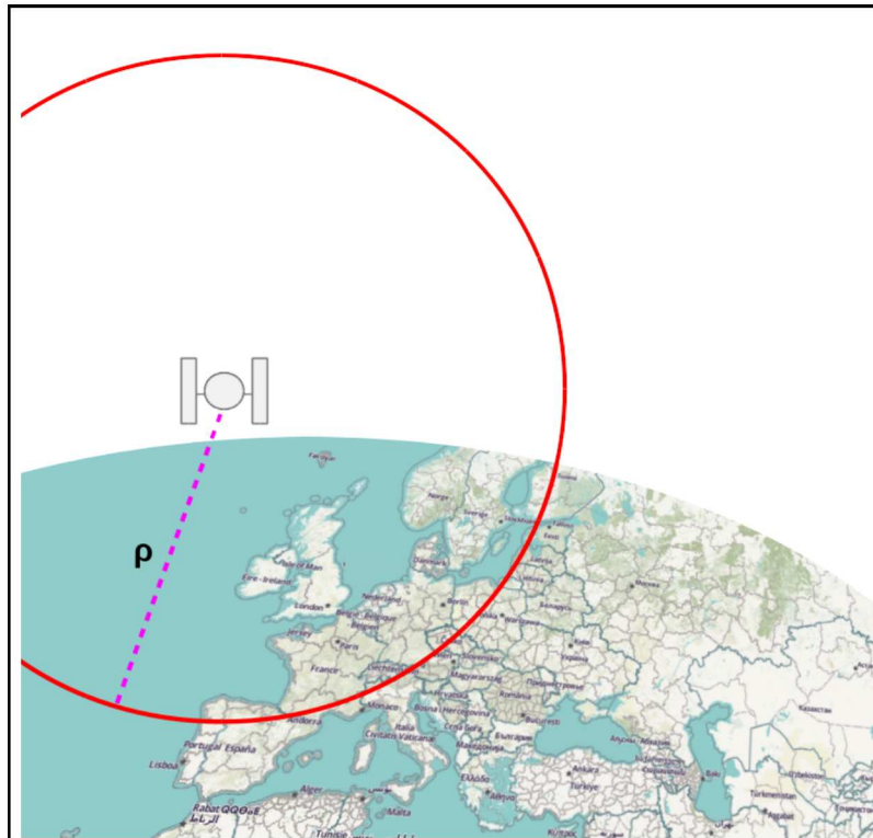
Figure 1.5 – The red line represents the sphere where can be a GNSS receiver distant \rho from the satellite in figure.
