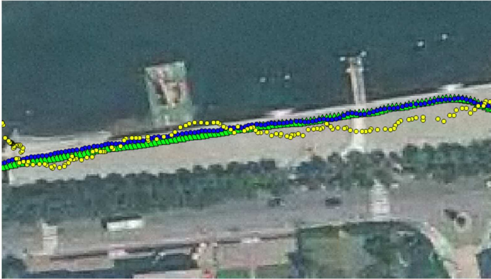
Figure 2.28 – Detail of the area in front of the lake with good exposition: points collected with geodetic receiver (green triangles), u-blox (blue circles) and smartphone (yellow circles) - Day 16-208
