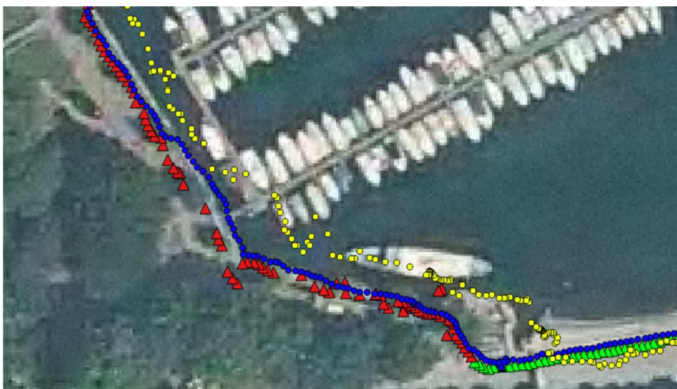
Figure 2.30 – Detail of an area with bad exposition: points collected with geodetic receiver (green triangles when the ambiguity solution was fixed, red triangles when it was not fixed), u-blox (blue circles) and smartphone (yellow circles) - Day 16-208
