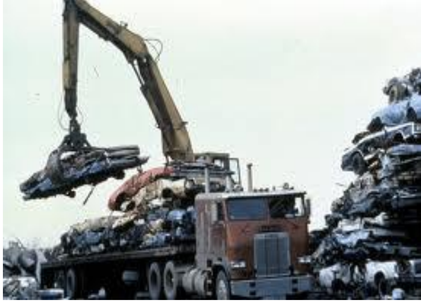
Figure 2-5 A crane loading auto bodies to be recycled from collection center(source: institute of scrap recycling industries)
