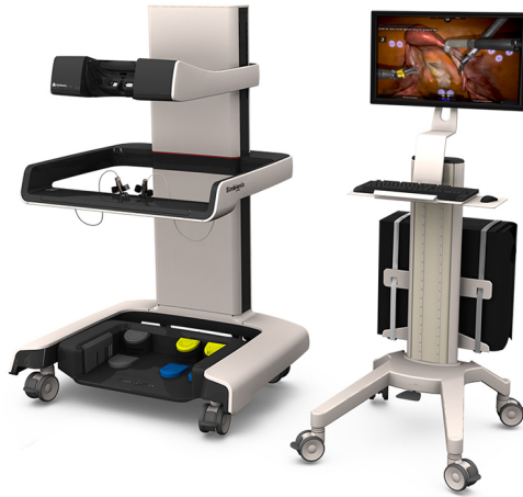
Figure 1.3: RobotiX Mentor surgical simulator: it is provided with an external screen, too, so that the instructor can easily give feedback to trainers.
