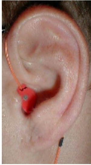
Figure 2.7: The position of Microphone in HRTF measurement [28]
