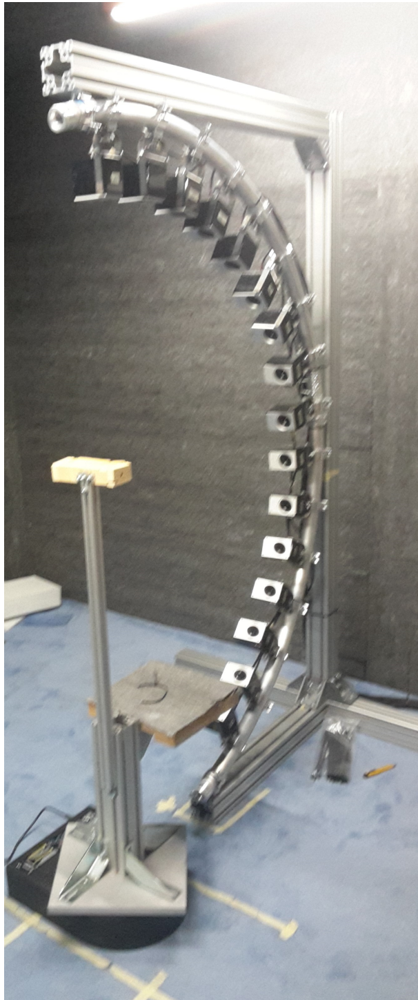
Figure 2.6: HRTF measurement setup at Sound and Music Computing (SMC) Lab, COMO, Polimi
