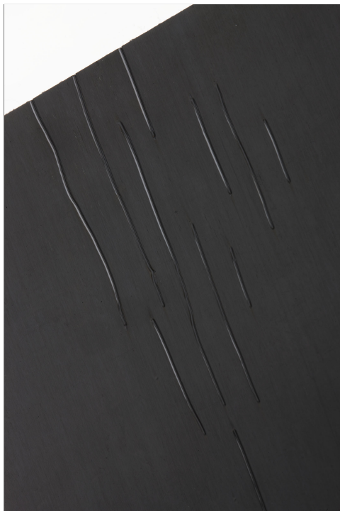
(a) Surface grooves caused by the initial use of a non-stick plastic sheet instead of release-film treated metal plates; trapped air bubbles caused the sheet ripples, that in turn caused these defects.
