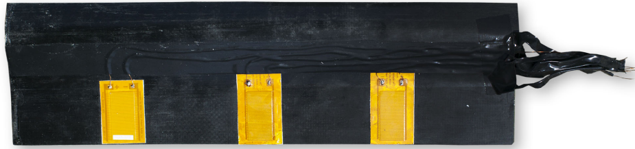
Figure 4.8: Photo of the first actuation system; the first actuator from the left has different overall size, since it is an earlier model, but the actuation force and the active section size are identical to the other two.
