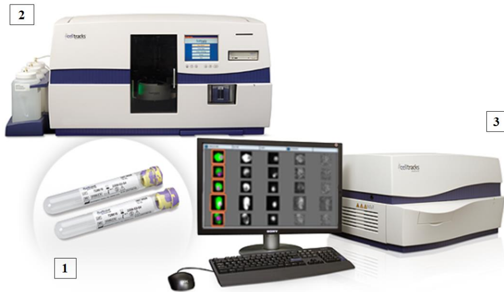
Figure 1.7: CellSearch™ System components. (1) CellSave Preservative tubes, in which blood is collected and stabilized for up to 96 h at room temperature, allowing the samples collection and the subsequent analysis in distant places. (2) Automated CELLTRACKS®AUTOPREP® System for the immunomagnetically cell enrichment and staining. (3) CELLTRACKS ANALYZER II® System for the selected cells automatic image generation 2 .
