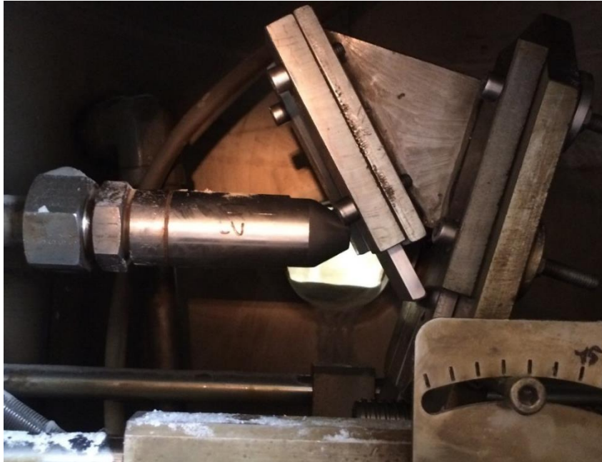
Fig. 27 60° configuration: the support is turned
