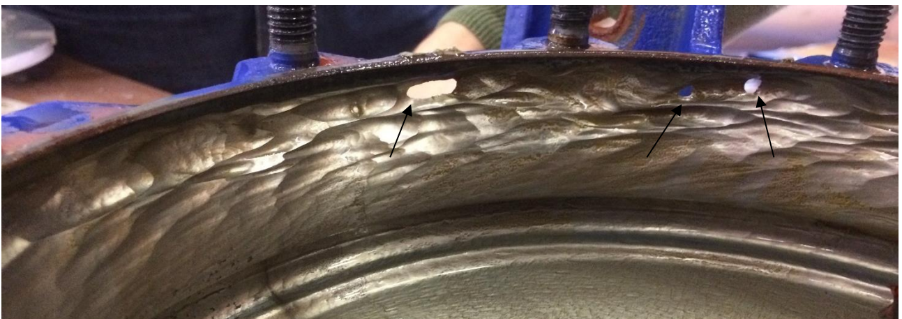
Fig. 20 Detail of the eroded pump: 3 holes on the volute casing.
