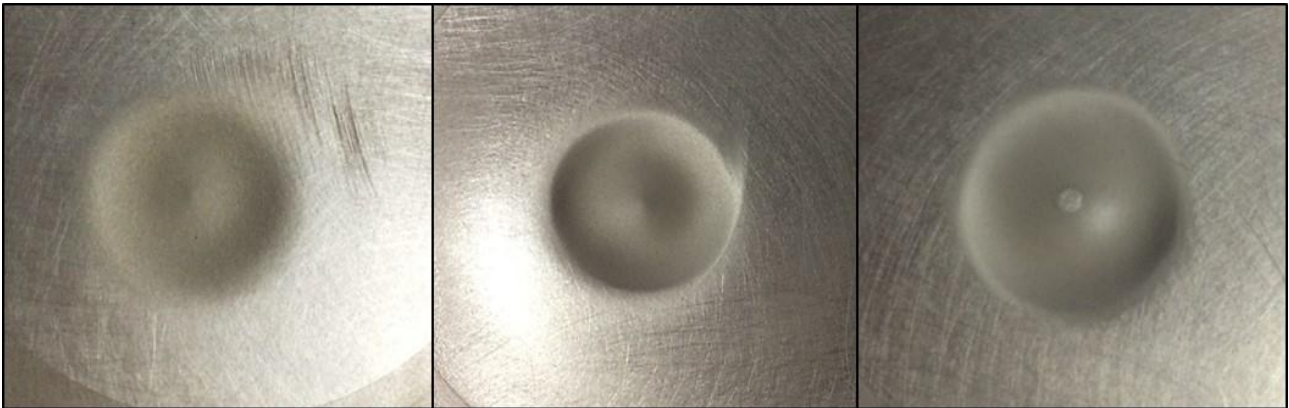
Fig. 59 Erosion Effect on AISI 410: from left to right impacted by large sand, medium and thin
