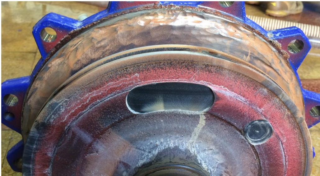
Fig. 22 Impeller and eroded casing
