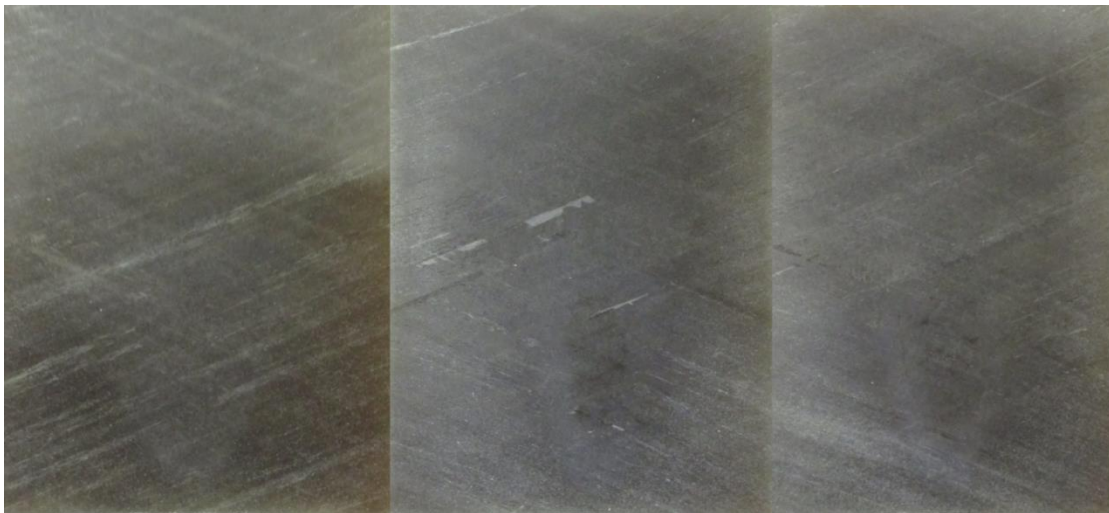
Fig. 63 Erosion effect, from right to left: 5, 15 and 30 minutes duration at 15° inclination
