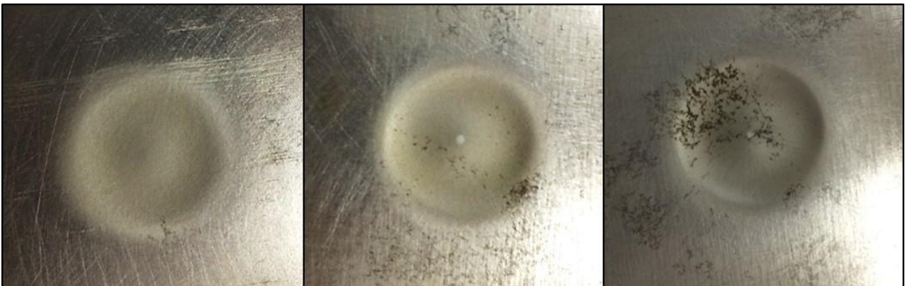
Fig. 60 Erosion Effect on AISI 4130: from left to right impacted by large sand, medium and thin
