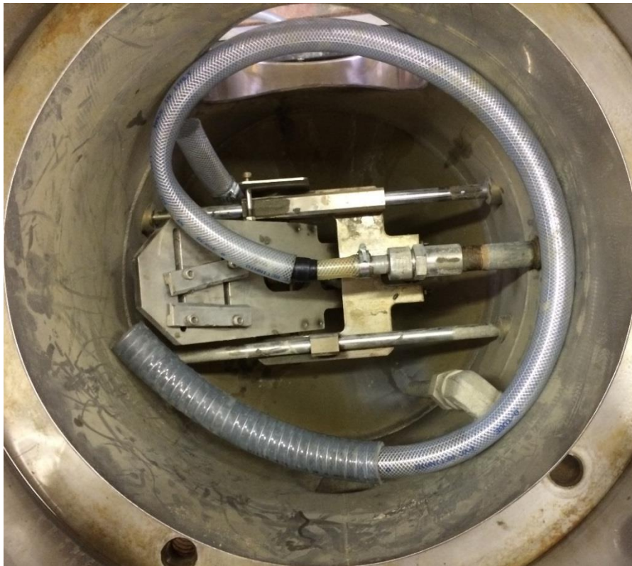
Fig. 31 First configuration in the filling set up: the tank is filled till the submersion of the nozzle
