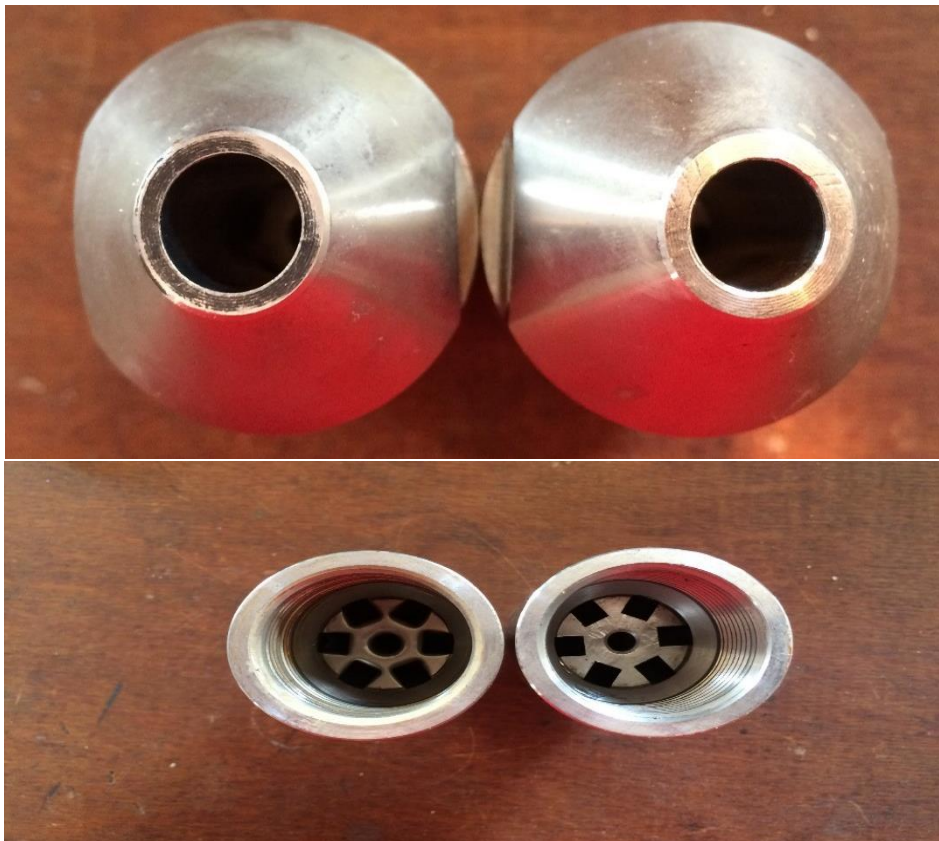
Fig. 93 Comparison of a used nozzle (left) and a new one (right)
