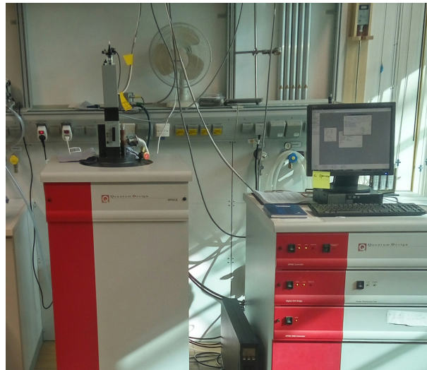
Figure 5.3: MPMS device used for the magnetic measurement characterization of the samples
