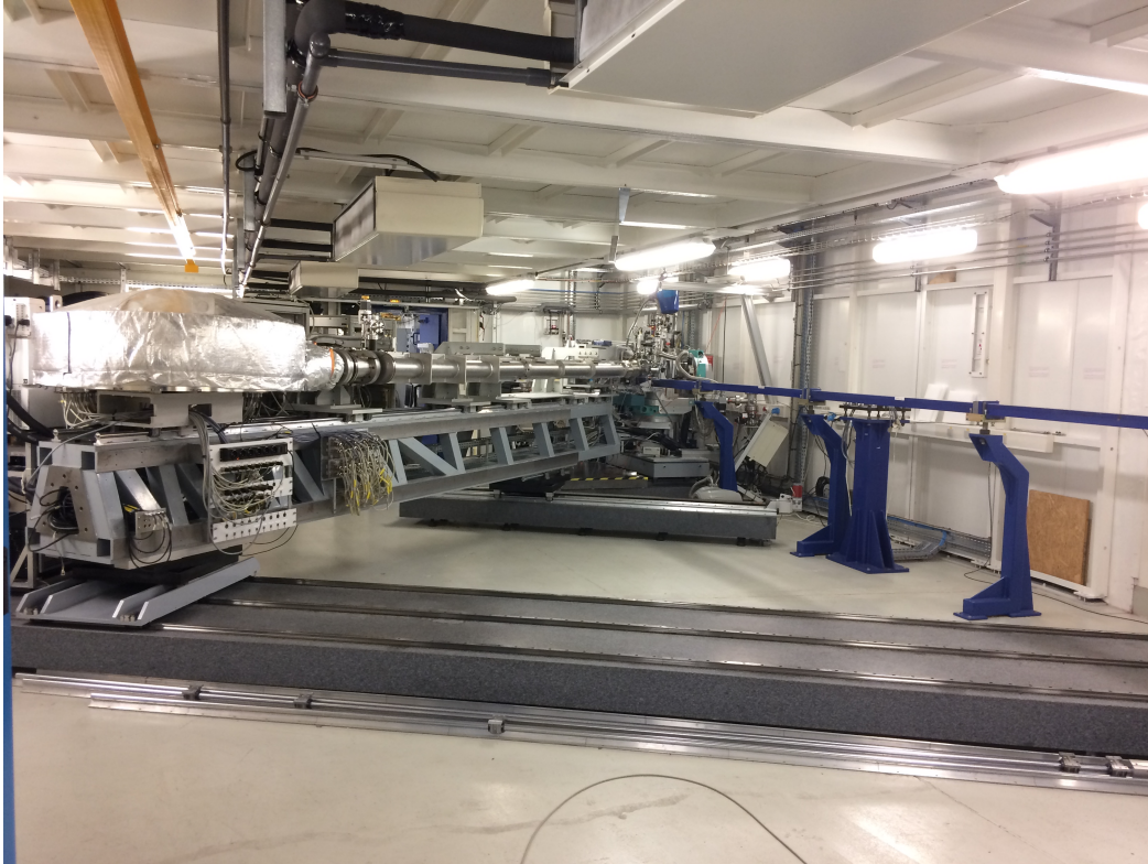
Figure 1.6: Photograph of the Main station setup. It is clearly visible the 7 m spectrometer arm where the analyzers are mounted.
