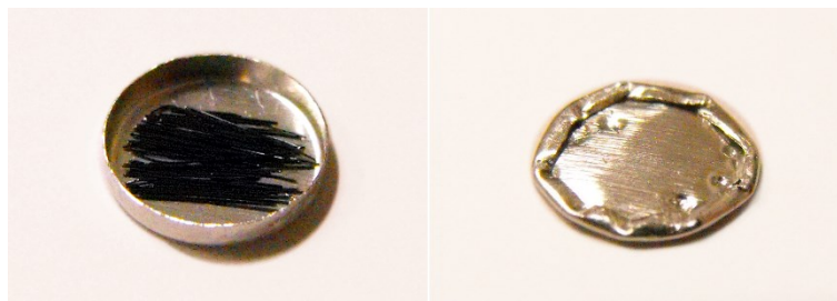
Figure 4-1 - Pan with layer of wires. Open on the left and then closed on the right.
