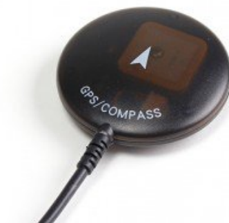
Figure 2.5: GPS receiver and compass module
