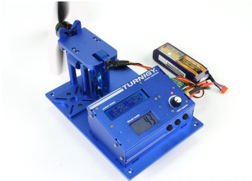
Figure 2.22: Turnigy thrust stand and power analyser
