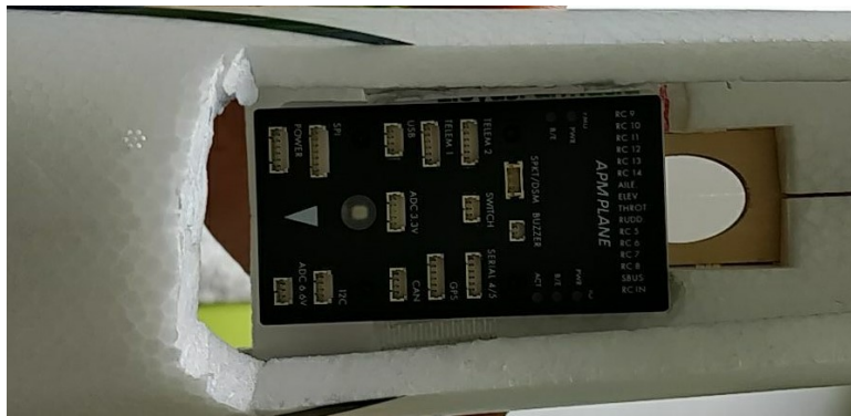
Figure 2.7: HKPilot32 mount inside the Bixler (bottom view)
