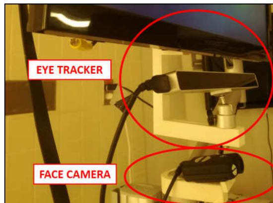
*Figure 3.16: Eye Tracker and Face camera with the respective supports.*
