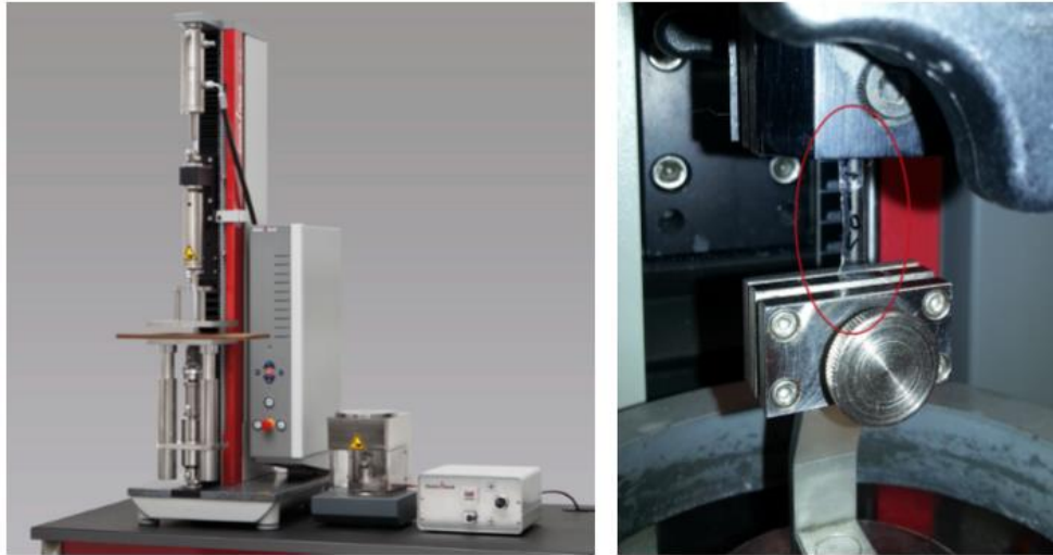
Figure 3.11 The Zwick Roellr Z 5.0 tensile machine used for the tensile tests on silicone samples (left) and (right) a dumb bell shaped sample during the experiment
