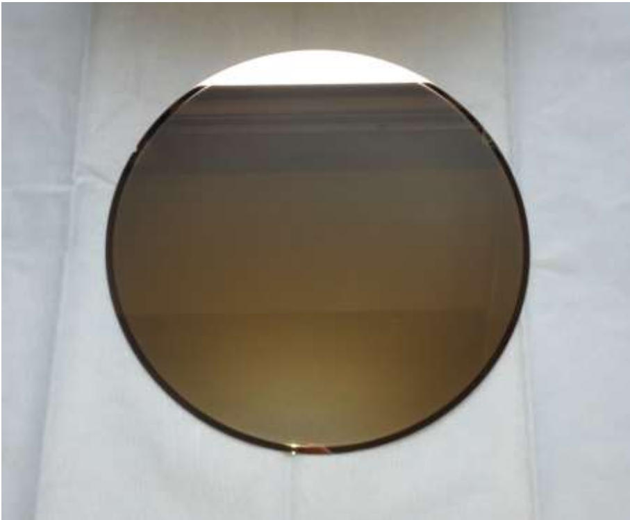
Image 52: Photograph of whole Au-plated wafer before processing
