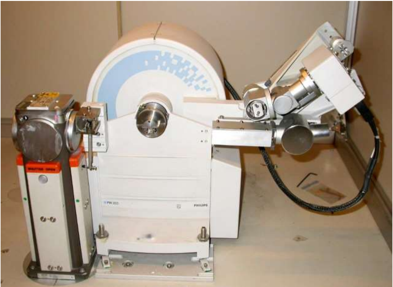
Image 65: Philips® X-pert PW1830® powder diffractometer
