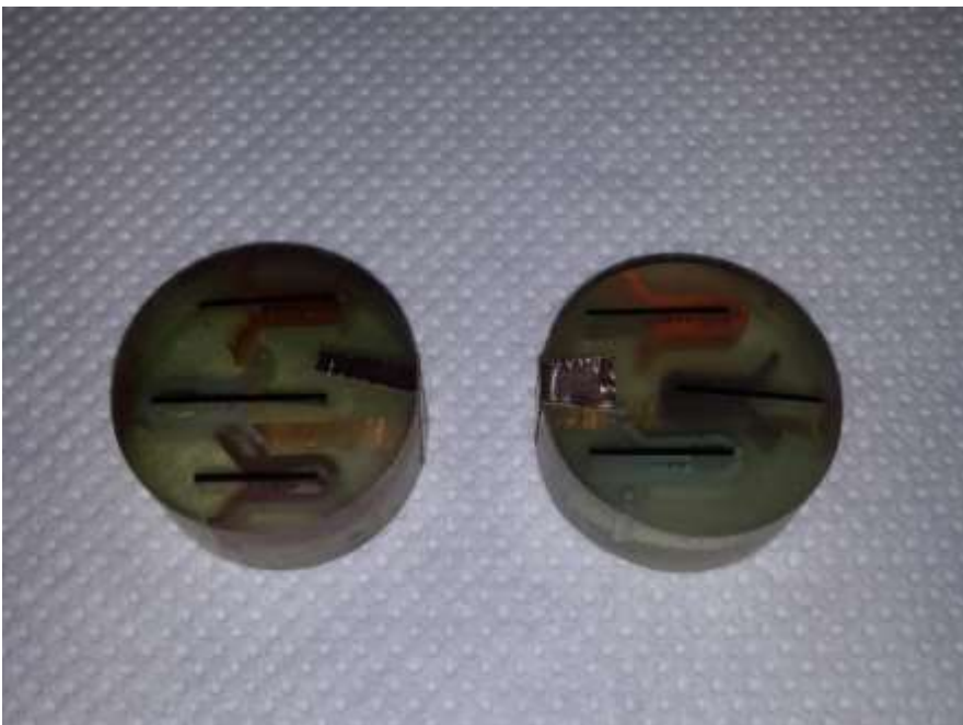
Image 36: Photograph of resin encased samples for section SEM testing
