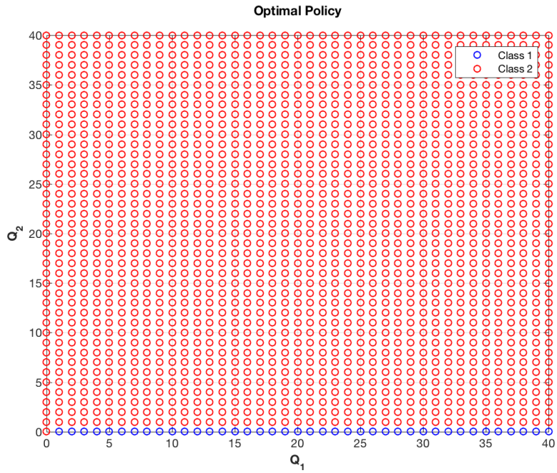
Figure 4.26: Policy iteration results for Class 2 zone, the parameters used are: \lambda_{11} = 23 , \lambda_{12} = 12 , \lambda_{21} = 6 , \lambda_{22} = 13 , \mu_1 = 100 , \mu_2 = 147 , c_1 = 1.4 , c_2 = 1 , N = 40 .
