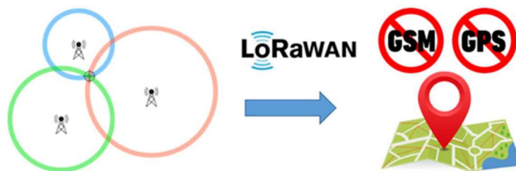
Fig. II-1. LoRaWAN geolocation. No GPS or GSM units were used.
