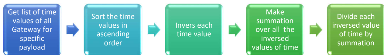
Fig.3-3. Basic process of weighting algorithm using time of arrivals
