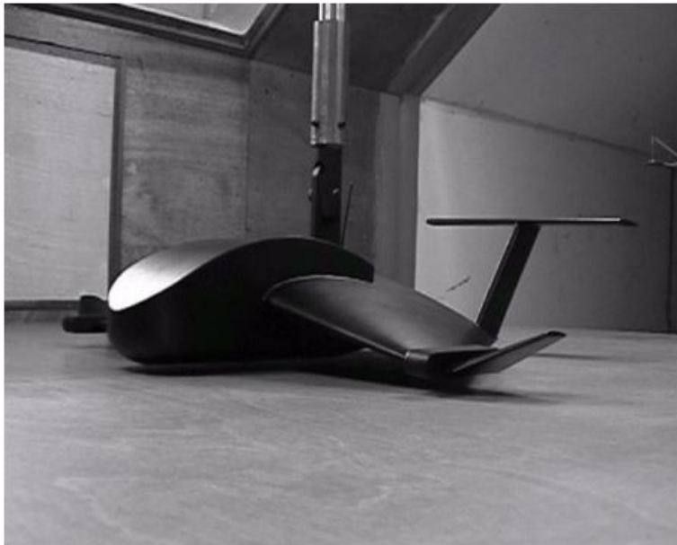
Figure 1.12: WIG craft model mounted in a wind tunnel. Reproduced with permission from [5].
