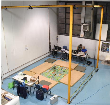
Figure 6.1: Photo of the cage with Optitrack cameras on top
