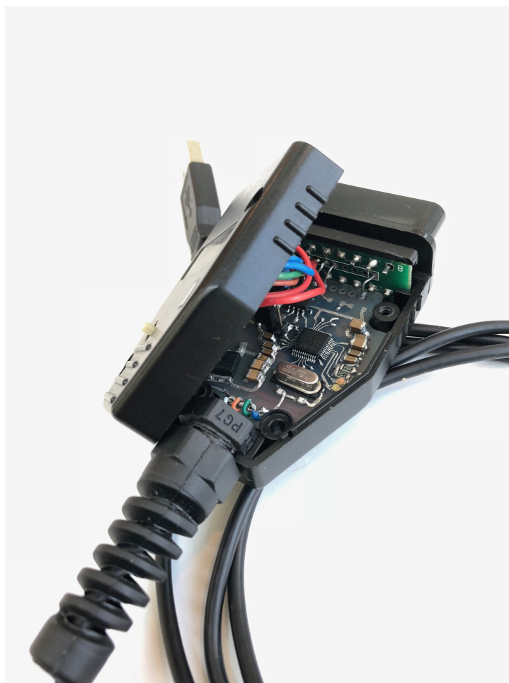
Figure 5.2: Final CANtact device
