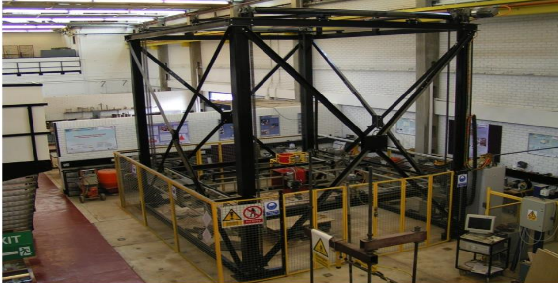
Figure 29. Concrete Printing Machine ( Lim et al, 2011 ).
