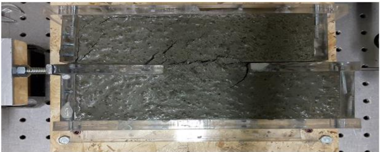
Figure 80. Shear Failure at 130mins.
