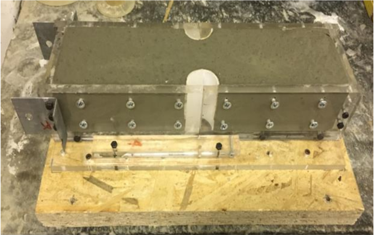
Figure 52. Full Tensile Testing Apparatus
