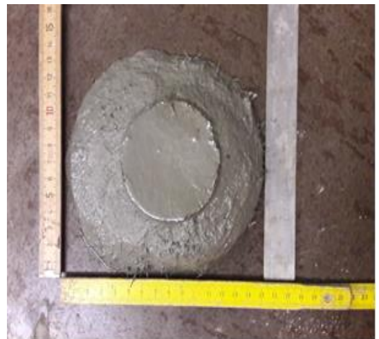
Figure 59. Performed Slump Test.
