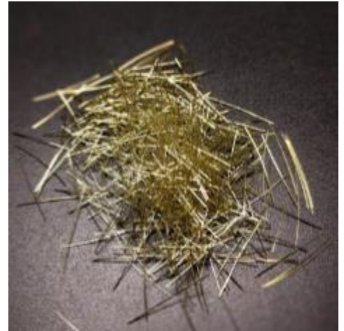
Figure 54. Steel Fibers (AZICHEM Ltd)
