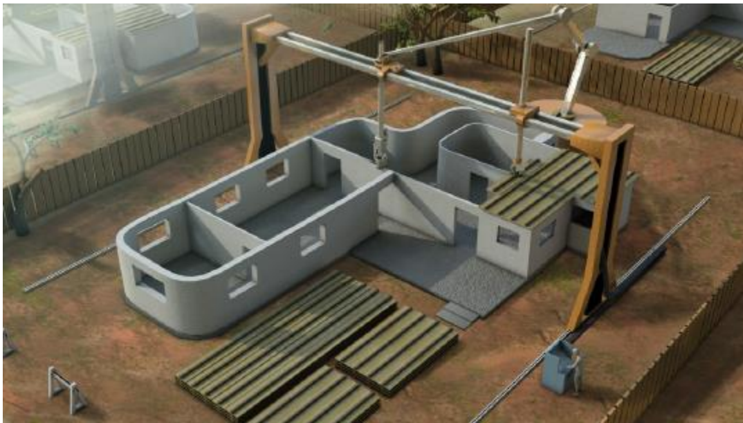
Figure 23. Multiple Outlet CC Printer Model ( contourcrafting.org, 2014 ).
