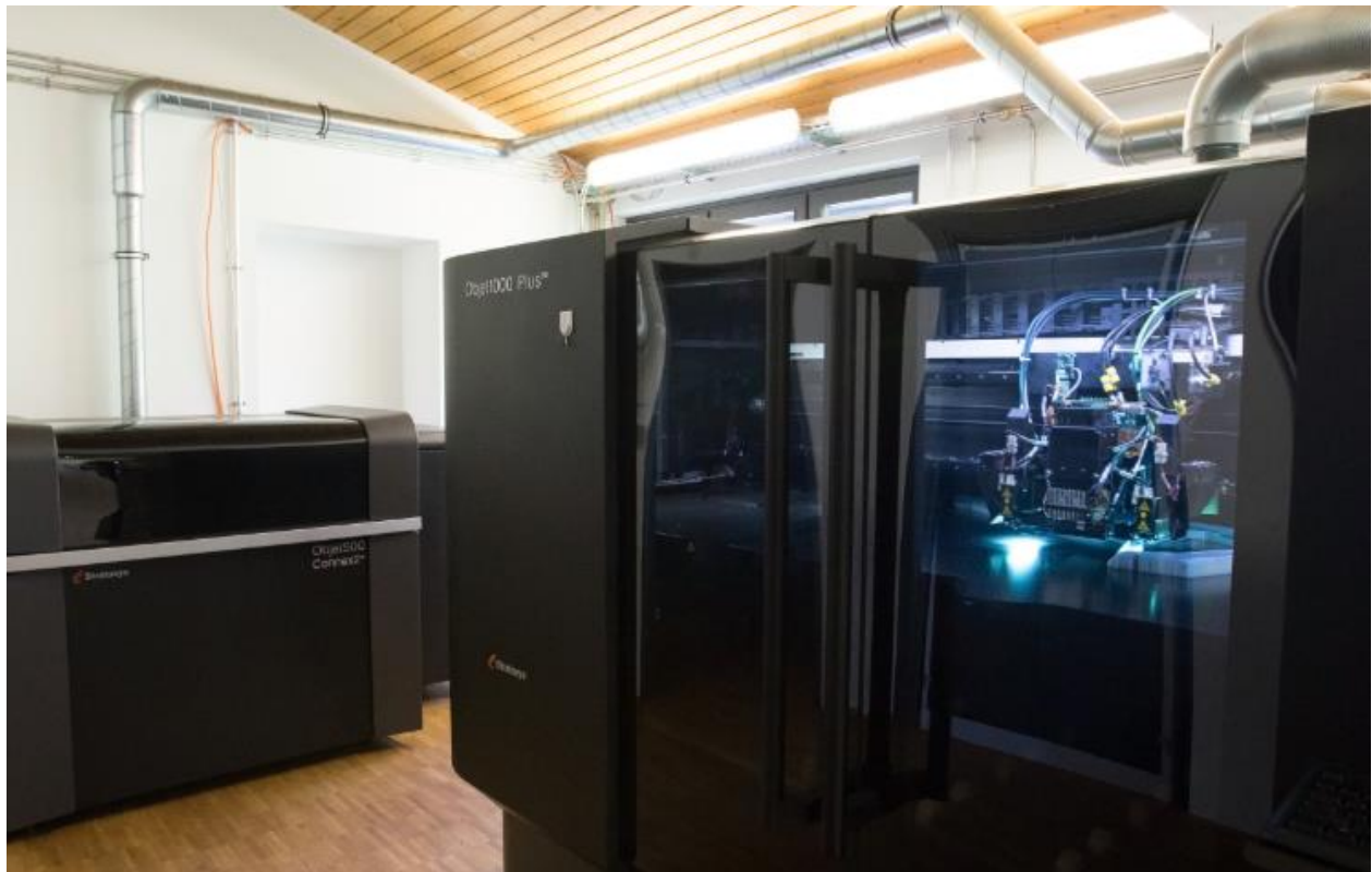
Figure 8. Material Jetting Printer ( 3dhubs.com )
