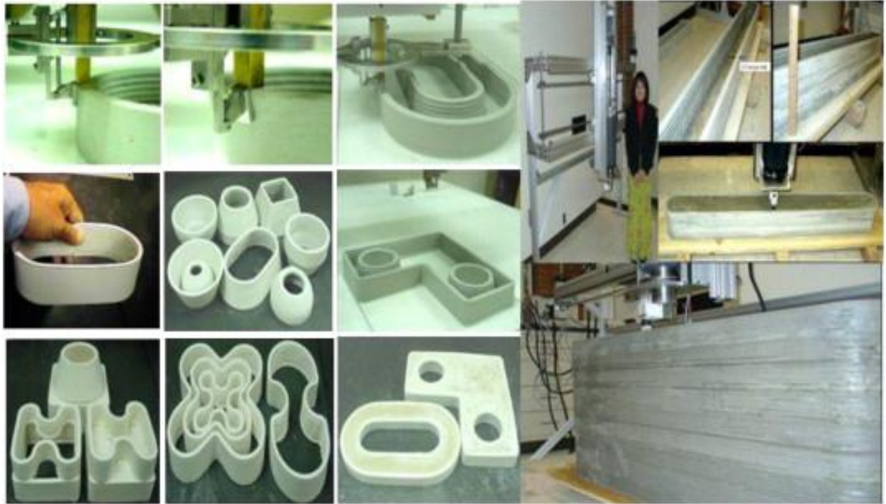
Figure 25. CC printed Structures and Machine (top right) (Lim et al, 2011).
