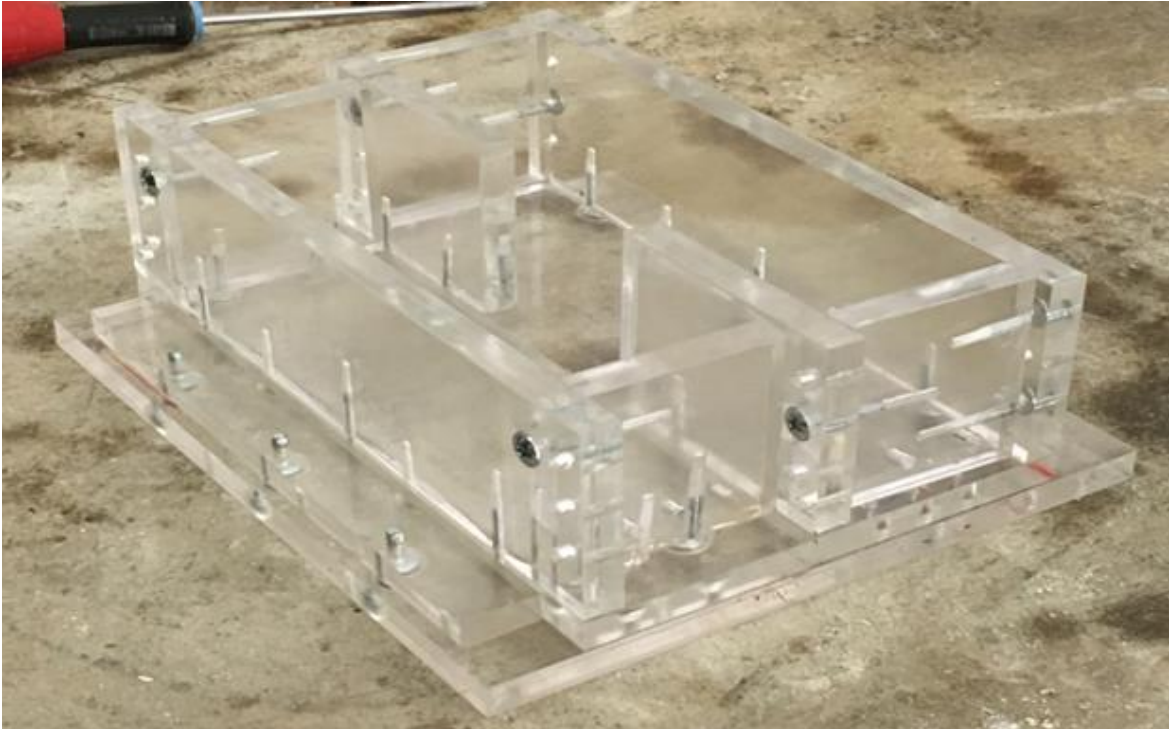
Figure 48. Empty Shear Testing Apparatus
