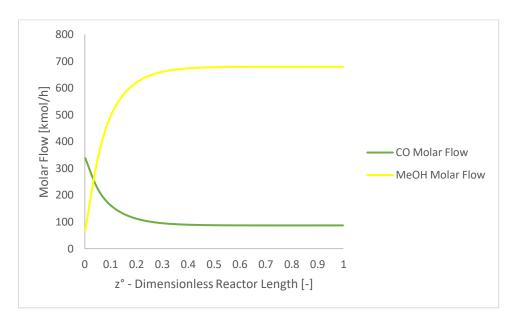
Figure 4.14 Methanol and CO molar flow inside the reactor at centerline, for the stream 2D adding 1300 kmol/h of  $H_2$ .
