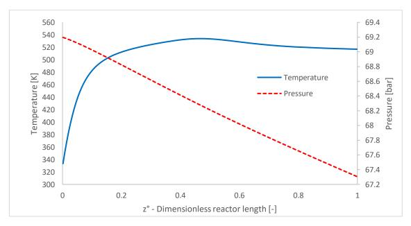
Figure 4.4 Temperature and Pressure profile at centerline vs reactor length for stream 2E with constant  $RI/N_T = 3.877$  kmol/h per each tube and  $T_{cool}$  decrease to 507.15 K. Blue solid line: Temperature, red dashed line: Pressure.
