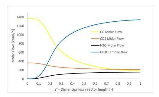
Figure 3.2 Molar flows inside the reactor.
