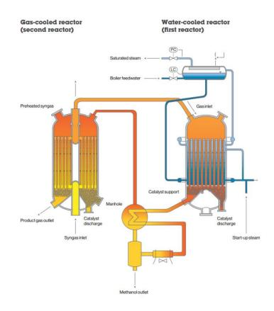
Figure 4.9 Lurgi configuration about methanol synthesis [53].
