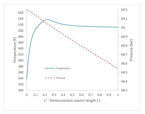
*Figure 3.3 Temperature and Pressure profile at centerline vs reactor length. Blue solid line: Temperature, red dashed line: Pressure.*
