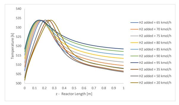
Figure 4.8 Temperature profile for a reactor with as fresh feed stream 2E and the addition of pure  $H_2$  after the mixing with the recycle.
