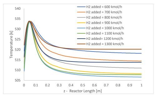
Figure 4.15 Temperature profile for a reactor with as fresh feed stream 2D and the addition of pure H2 after the mixing with the recycle.
