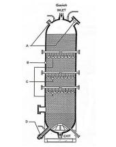
Figure 1.8 Design of a Quench reactor [15].
