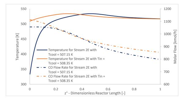
Figure 4.5 Temperature and CO molar flow for simulation with as fresh feed stream 2E. Blue line:  $T_{cool} = 507.15$  K and Tin = 323 K; Orange line:  $T_{IN} = T_{cool} = 508.35$  K: Continue line: Temperature [K]; Dashed line: CO molar Flow [kmol/h].
