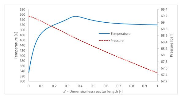
Figure 4.3 Temperature and Pressure profile at centerline vs reactor length for stream 2E with constant  $RI/N_T$  = 3.877 kmol/h per each tube. Blue solid line: Temperature, red dashed line: Pressure.
