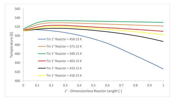
Figure 4.12 Temperature profile of the second reactor for a Lurgi configuation with as fresh feed stream 2E.
