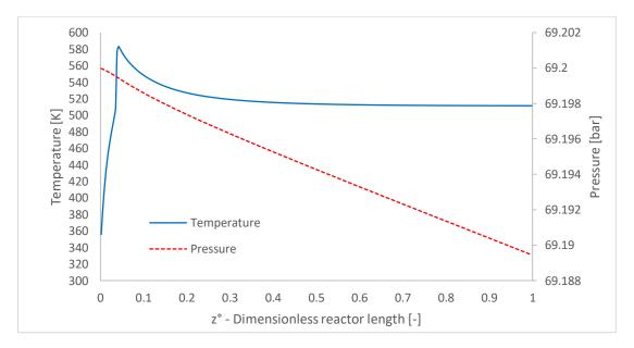
Figure 4.1 Temperature and Pressure profile at centerline vs reactor length for stream 2E with constant  $N_T$  = 4650. Blue solid line: Temperature, red dashed line: Pressure.
