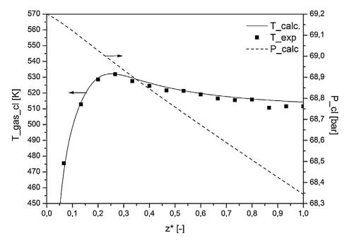
Figure 3.4 Temperature and Pressure profile from Montebelli et al. [7].
