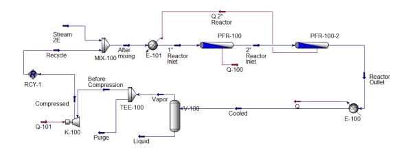
Figure 4.10 Lurgi Methanol synthesis loop in Aspen HYSYS V 8.8.
