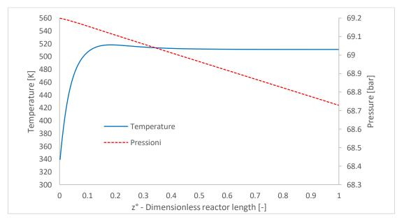
*Figure 3.5 Temperature and Pressure profile at centerline vs reactor length for the improved model. Blue solid line: Temperature, red dashed line: Pressure.*
