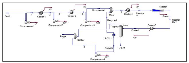
Figure 2.1 Methanol Synthesis loop in Aspen HYSYS V8.8.
