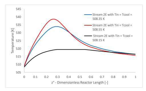
Figure 4.6 Temperature profile at centerline vs reactor length for stream 2E with  $N_T$  = 708. Blue solid line:  $T_{IN}$  =  $T_{cool}$  = 508.35 K, Red solid line:  $T_{IN}$  =  $T_{cool}$  = 508.55 K, Black solid line:  $T_{IN}$  =  $T_{cool}$  = 508.15 K.
