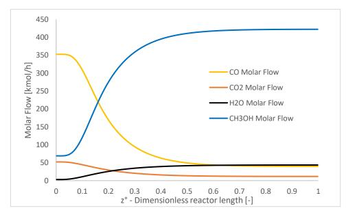
*Figure 3.6 Molar flows inside the reactor for the improved model.*
