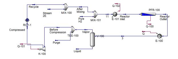
Figure 4.7 Synthesis loop when a pure H2 stream is added to the fresh feed mixed with the recycle.
