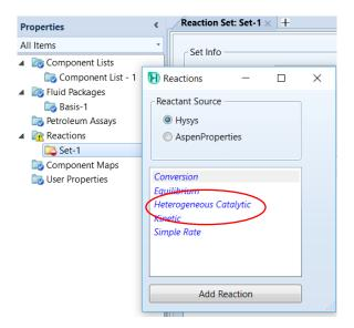
Figure 2.11 Reaction set attachment.
