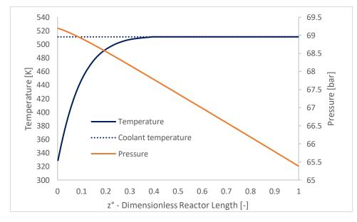
Figure 4.13 Temperature and Pressure profile at centerline vs reactor length for stream 2D with constant RI/NT = 3.877 kmol/h per each tube . Blue solid line: Temperature, blue pointed line: Tcool, red solid line: Pressure.
