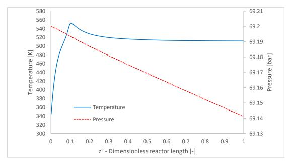
Figure 4.2 Temperature and Pressure profile at centerline vs reactor length for stream 2E with constant  $N_T$  = 4650 and flow ratio = 0.9995. Blue solid line: Temperature, red dashed line: Pressure.
