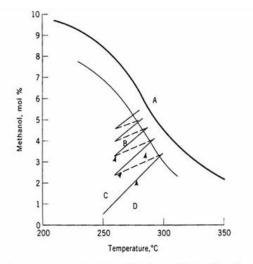
Figure 1.7 Profile of Methanol conversion vs Temperature for a Quench reactor [17].
