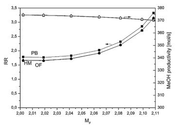
Figure 1.5 Methanol productivity and Recycle Ratio vs  $M_F$  [7].
