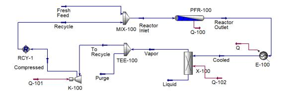
Figure 3.1 Methanol synthesis loop [7].
