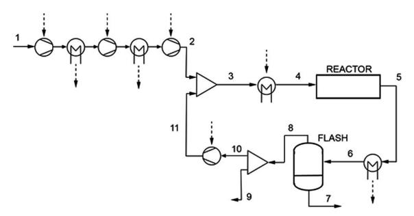
Figure 1.4 Methanol Synthesis Loop [6].
