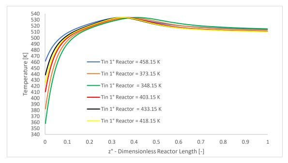
Figure 4.11 Temperature profile of the first reactor for a Lurgi configuration with as fresh feed stream 2E.
